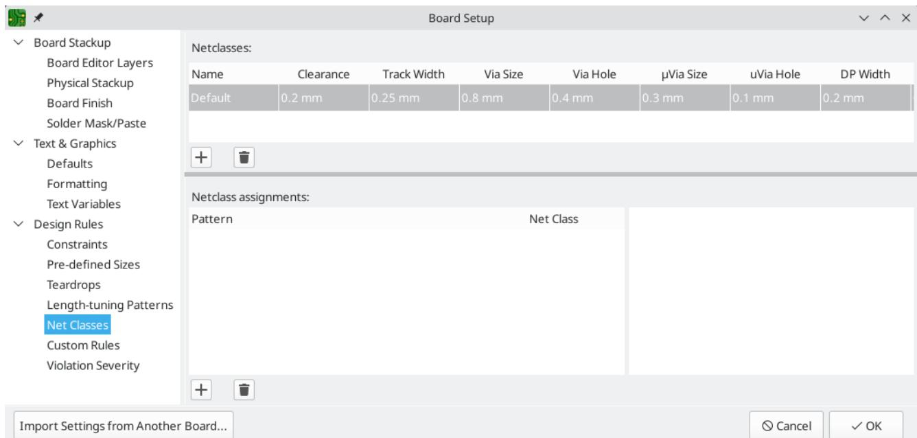
Track width and spacing can be managed manually by the designer during layout, but net classes are recommended because they provide an automatic way to manage and check design rules.
