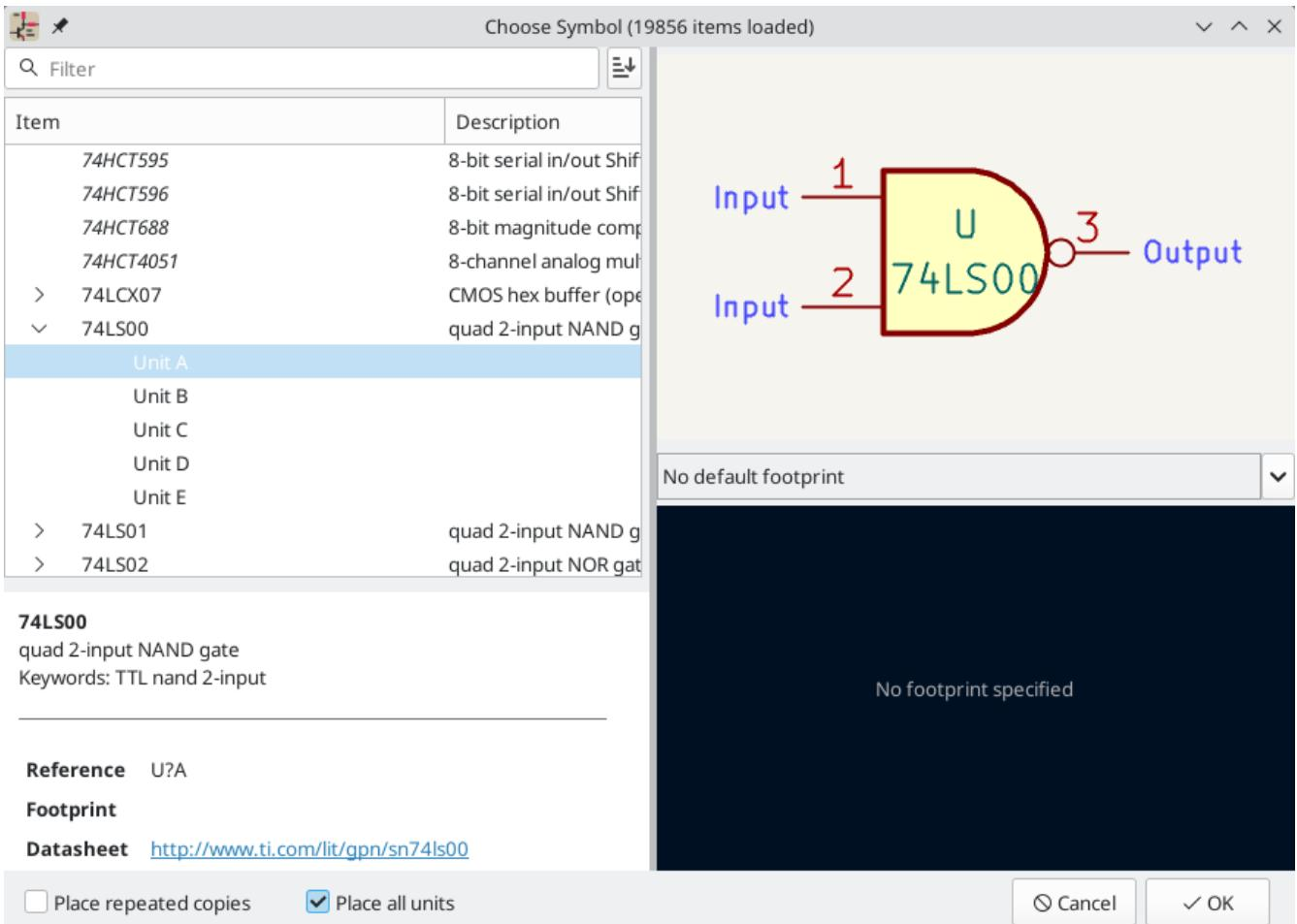
By default, only the symbol/library name and description columns are shown. Additional columns can be added by right-clicking the column header and selecting **Select Columns**.
