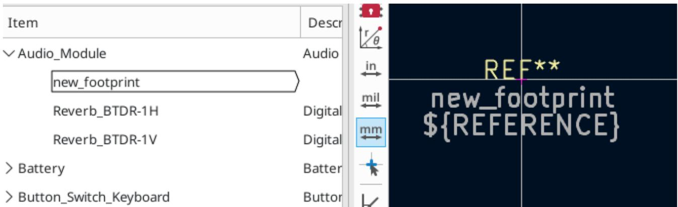
These items are centered on the footprint's anchor (origin point), which is indicated with a magenta cross symbol. The anchor can be repositioned (changing the (0, 0) point for the footprint) by selecting the
