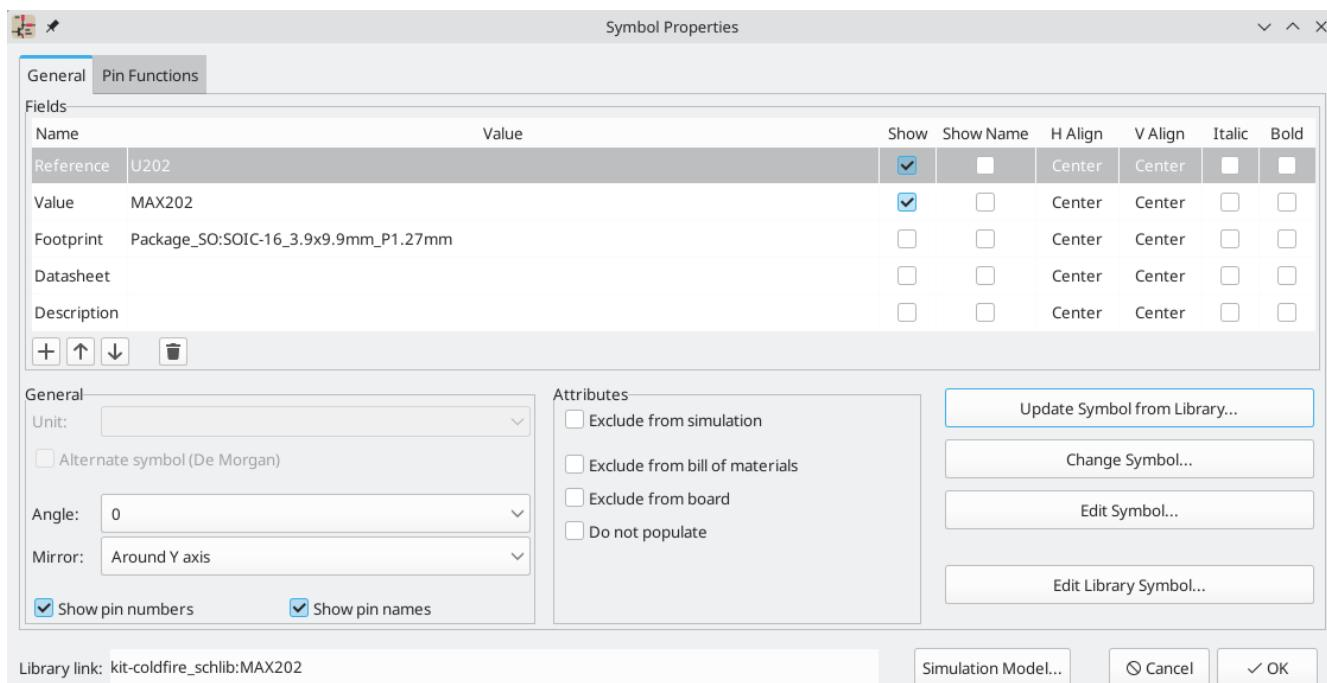
You can only use the properties dialog to edit one item at a time. To edit multiple items, use the properties manager, described below. There are also other tools that can be used to edit specific types of objects in bulk, such as the [Edit Text and Graphics tool](#) for editing text, labels, and graphic shapes, or the [Symbol Fields Table](#) for editing symbol fields in bulk.
