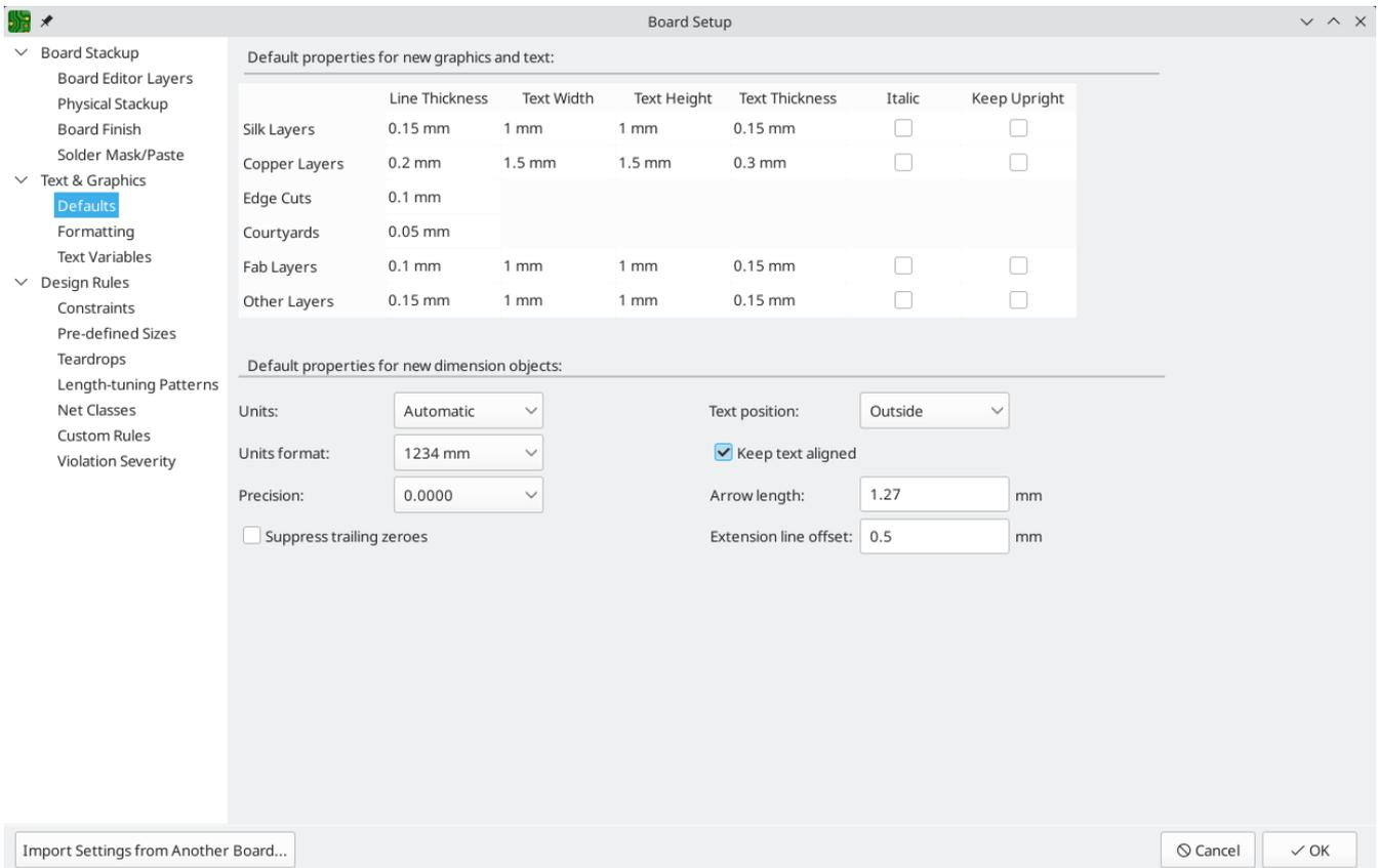
Line thickness, text size, and text appearance can be configured for the six different categories of layers shown in the dialog. Additionally, the properties for dimension objects can be configured for all layers. For more details about dimension properties, see the Dimensions section below.
