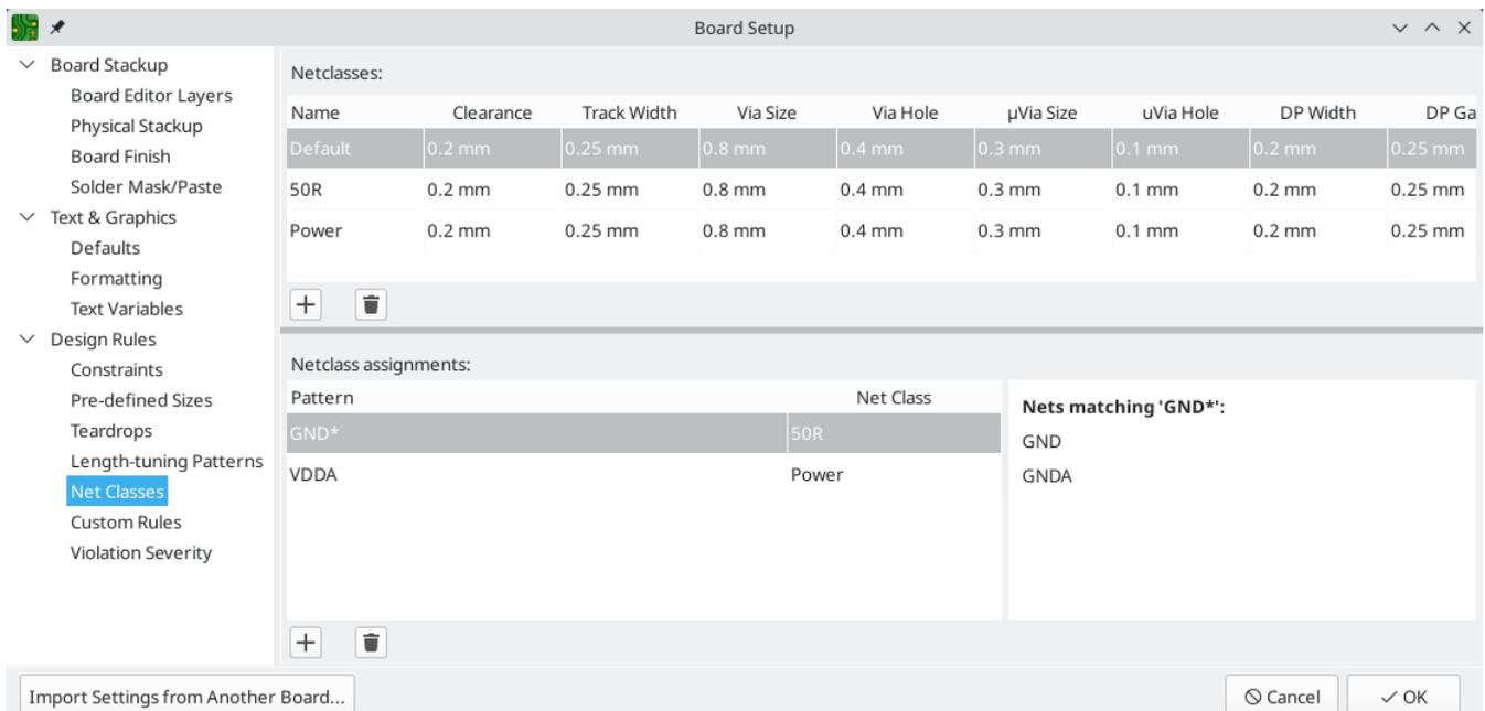
The upper portion of the Net Classes section contains a table showing the net classes in the design and the design rules that apply to each net class. Every class has values for copper clearance, track width, via sizes, and differential pair sizes. These values will be used when creating tracks and vias unless a more specific rule overrides them (see Custom Rules below).
