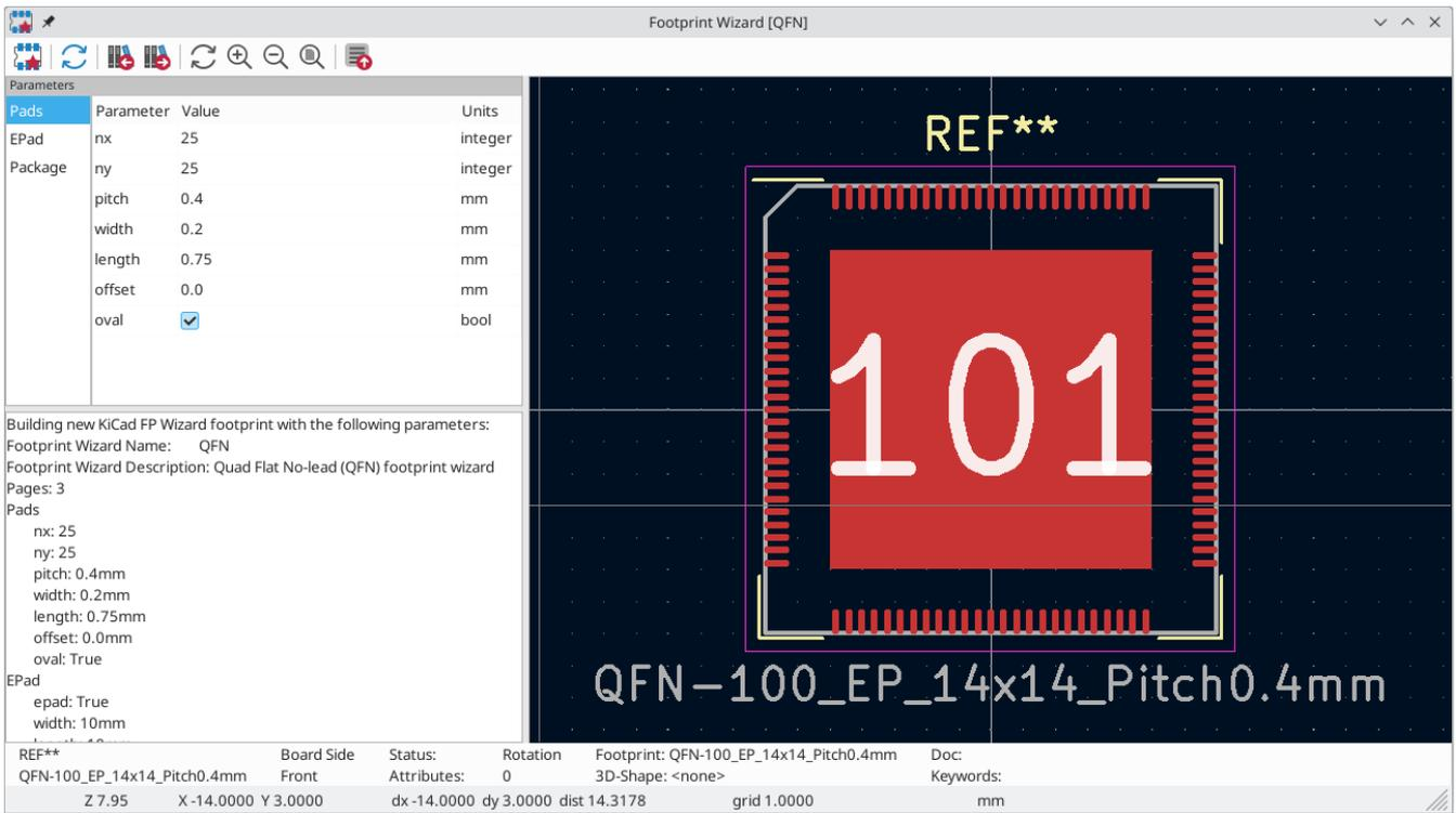
In the window that appears, fill out the parameters as appropriate. When the parameters are correctly filled out, press the
