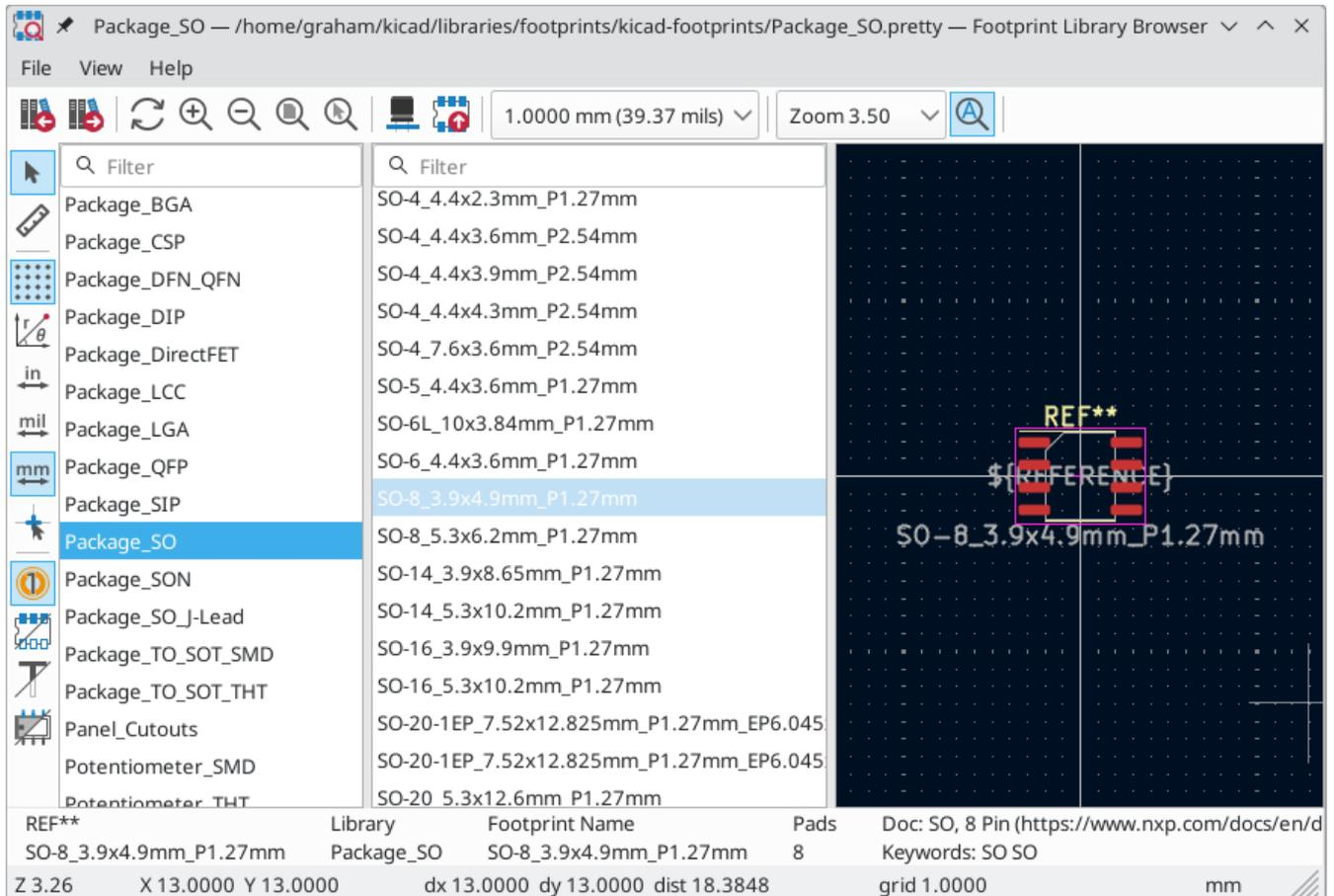
Double clicking the name of a footprint or using the
