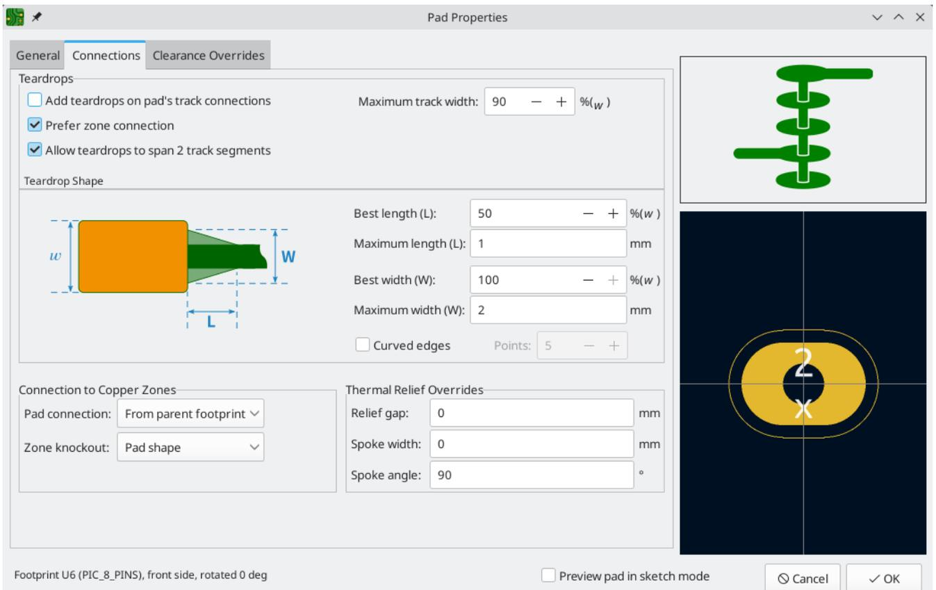
Teardrops in KiCad are small zones, meaning that when they refill they avoid shorting to copper objects on other nets. They are initially filled when they are added, but they are unfilled and refilled with other zones on the board: when using the Unfill All Zones and Refill All Zones commands, running DRC, generating fabrication outputs, etc. Teardrops can be shown in filled or outline mode using the zone display controls in the left toolbar.
