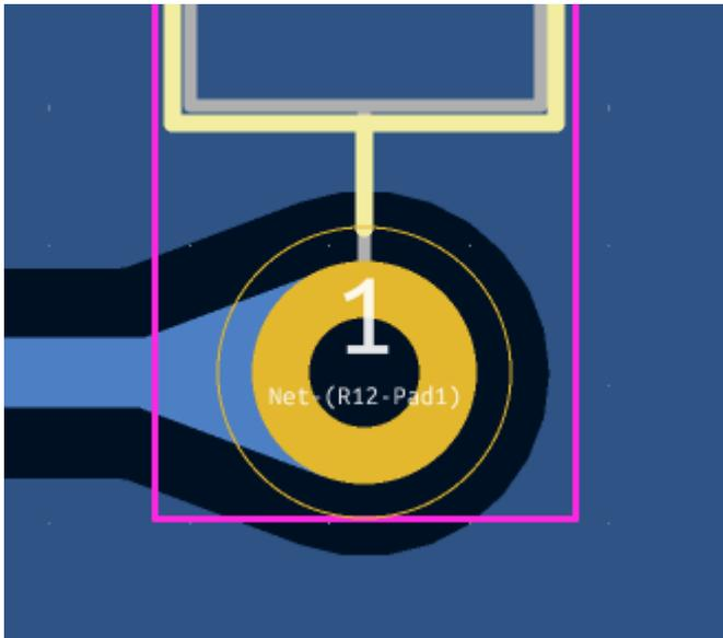
You can add teardrops to your design in bulk using the **Edit** → **Edit Teardrops...** dialog. This dialog has controls for filtering which objects are affected and settings for configuring the shape of the new teardrops. It also lets you edit or remove existing teardrops.
