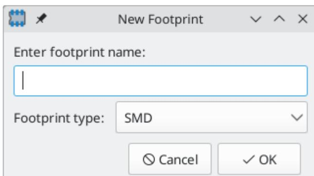
The name will set the name of the footprint, which is used when assigning a footprint to a symbol, and is also used as the filename of the footprint file on disk.
