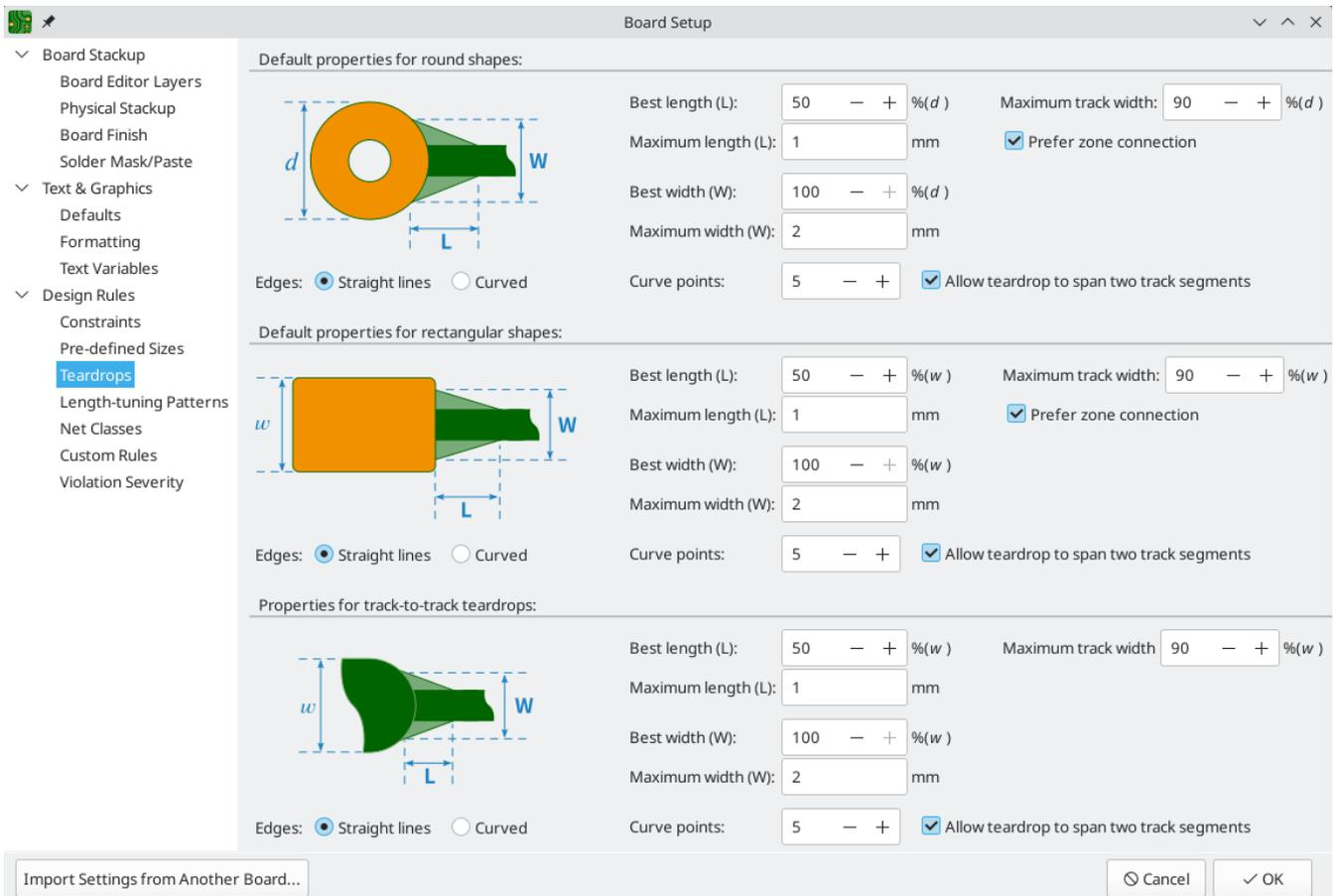
Rather than in bulk, you can add or edit teardrops for individual vias in the properties dialog for that via, or for individual pads in the **Connections** tab of the pad's properties dialog. The settings in the properties dialogs are the same as in the Edit Teardrops dialog. You can also edit teardrops for individual pads and vias with the Properties Manager.
