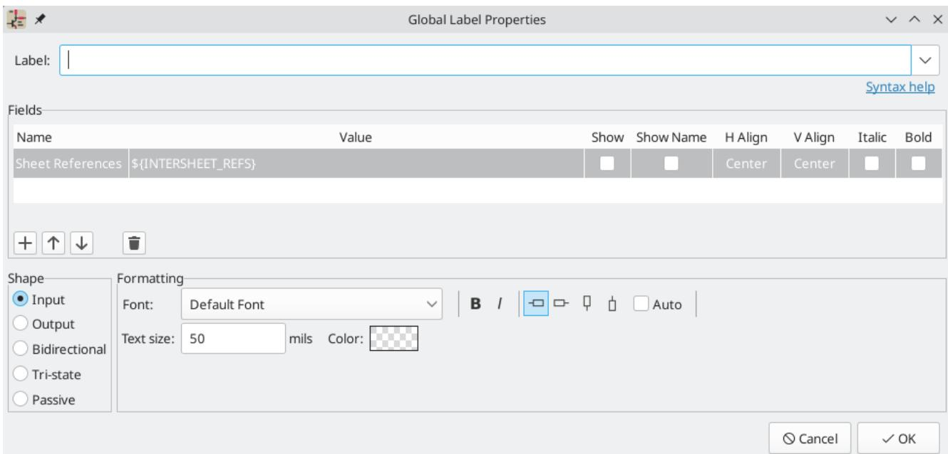
The **Label** field sets the label's text, which determines the net that the label assigns to its attached wire. Label text supports [markup](#) for overbars, subscripts, etc., as well as [variable substitution](#). Use the [Syntax help](#) link in the dialog for a summary.
