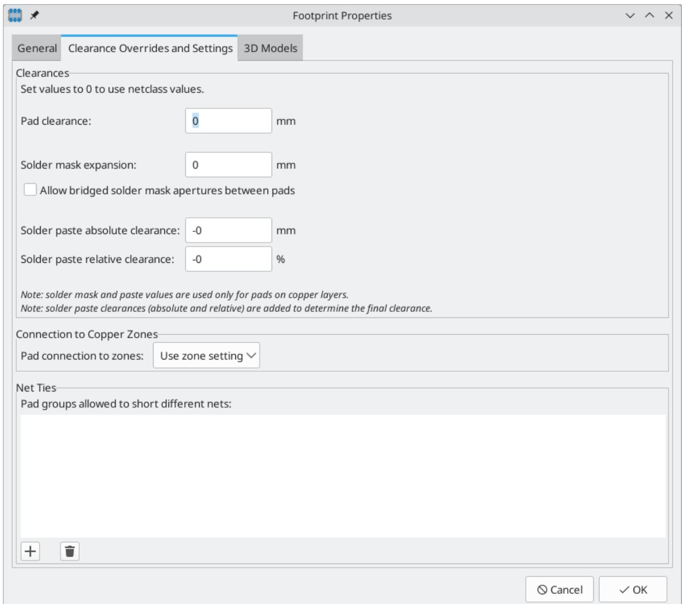
The screenshot shows the 'Footprint Properties' dialog box with the 'Clearance Overrides and Settings' tab selected. The dialog has three tabs: 'General', 'Clearance Overrides and Settings', and '3D Models'. The 'Clearances' section contains the following settings:
