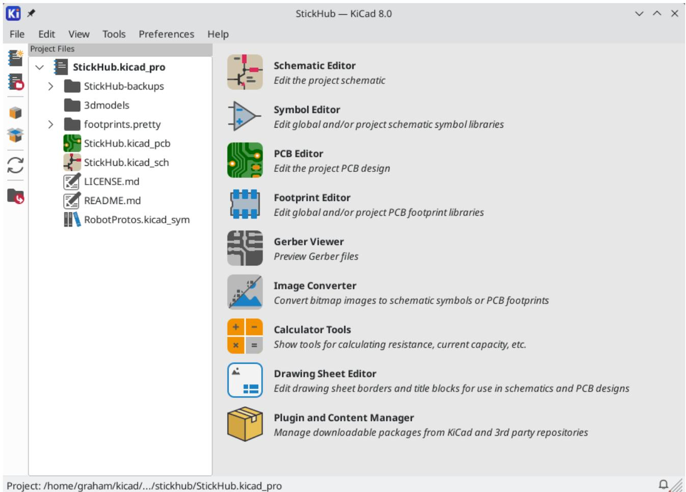
The KiCad project manager window is composed of a tree view on the left showing the files associated with the open project, and a launcher on the right containing shortcuts to the various editors and tools.
