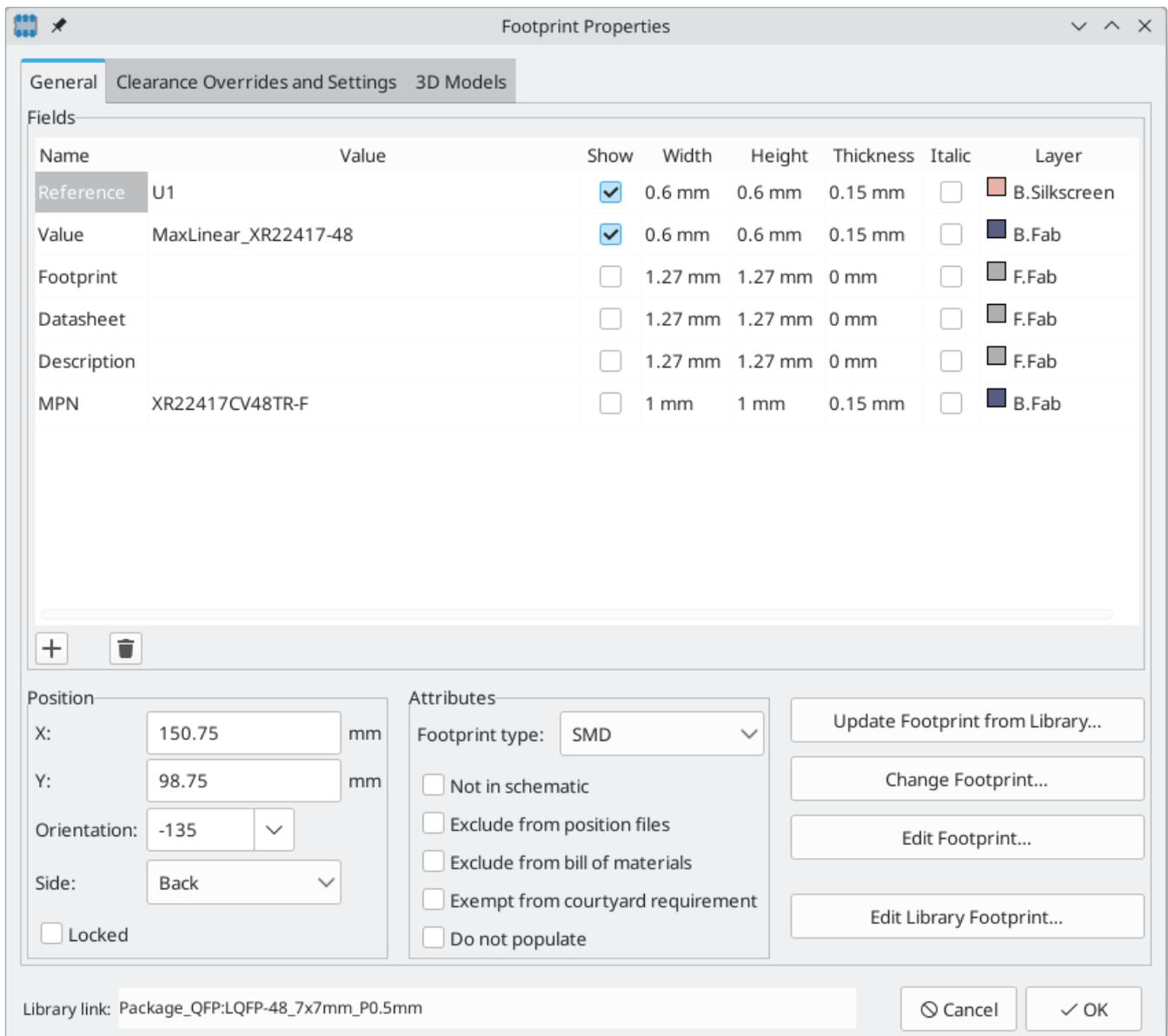
The majority of the settings in this dialog are the same as in the [footprint editor](#). You can edit the footprint's fields, attributes, clearance and zone connection settings, and 3D models, as in the footprint editor. However, here you can also set the footprint's position, orientation, and side. You can also update the footprint from the library, exchange it for a different footprint, or edit the footprint itself in the footprint editor.
