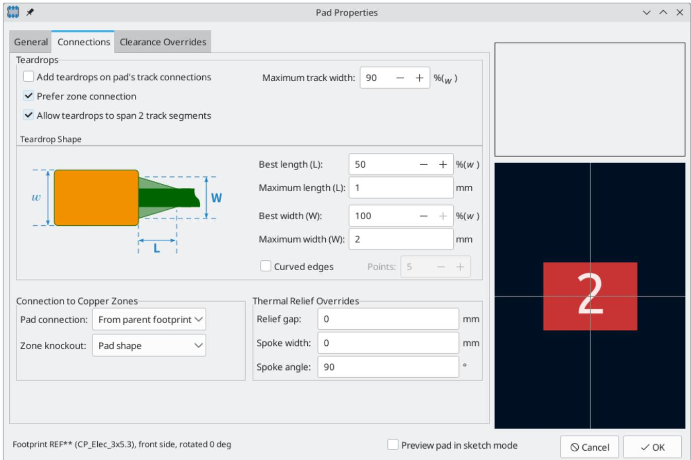
The Teardrops section contains settings controlling teardrop connections between tracks and the pad, if teardrops are used. Teardrop settings are explained in the [teardrop documentation](#).
