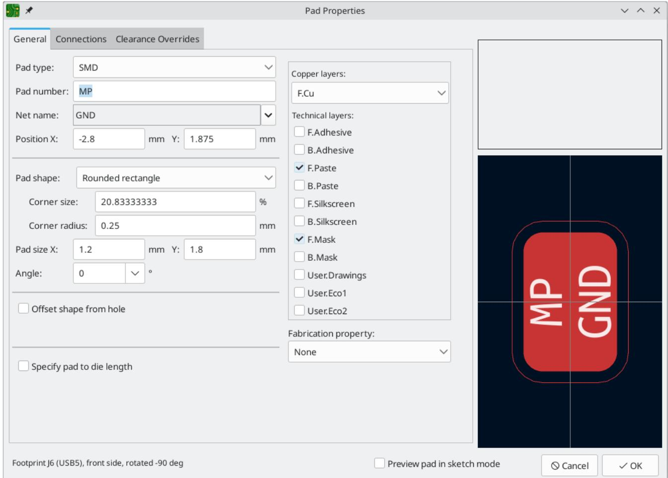
This dialog lets you edit the physical properties of the pad, including size and shape. You can also modify how the pad connects to other objects on the board, including clearance properties, teardrops, and thermal reliefs.
