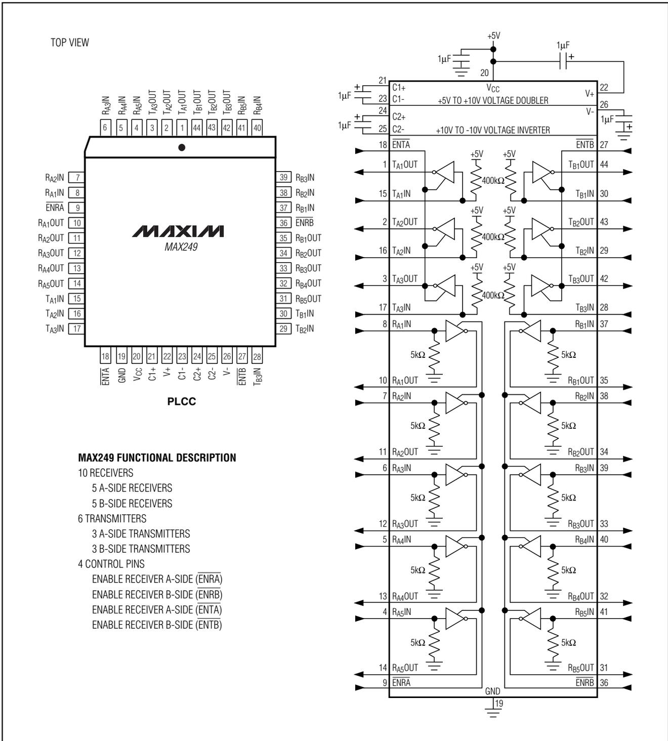
Figure 25. MAX249 Pin Configuration and Typical Operating Circuit
