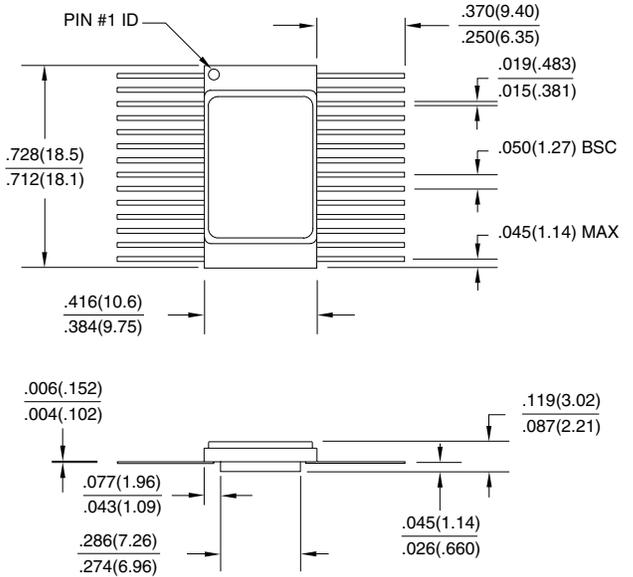
**32J**, 32-lead, Plastic J-ledged Chip Carrier (PLCC)
