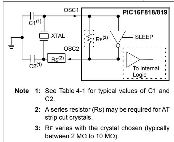
**TABLE 4-1: CAPACITOR SELECTION FOR CRYSTAL OSCILLATOR (FOR DESIGN GUIDANCE ONLY)**
