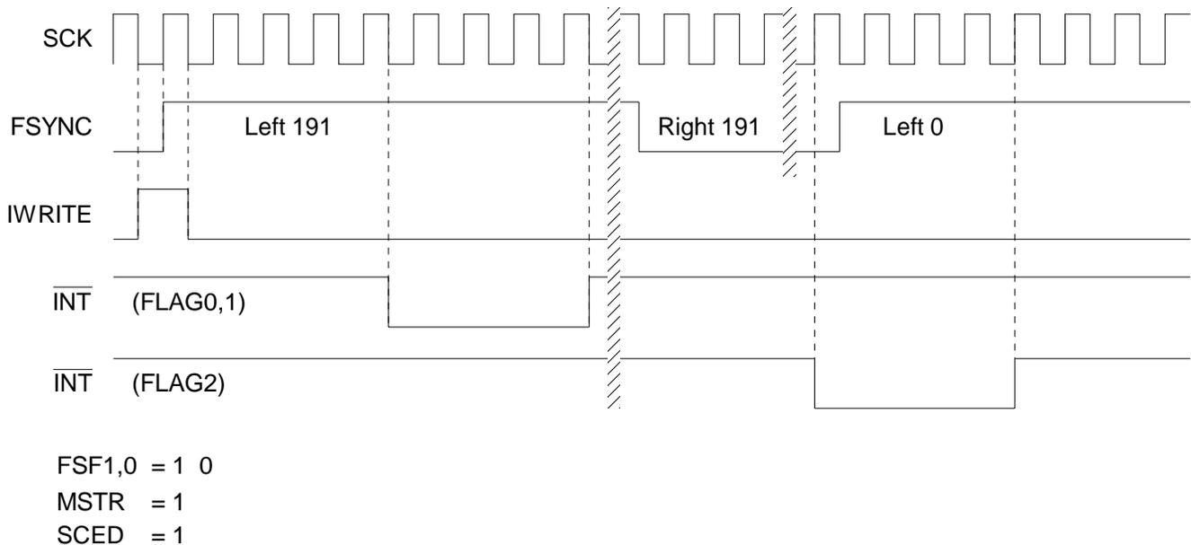
Figure 15. RAM/Buffer - Write and Interrupt Timing
