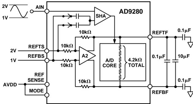
Figure 21. External Reference Mode—1 V p-p Input Span
