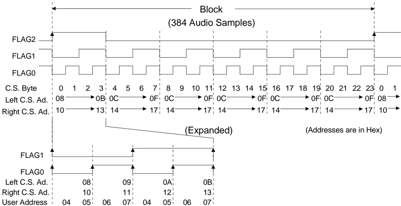
**Figure 14. CS8413 Buffer Memory Write Sequence - MODE 2**
