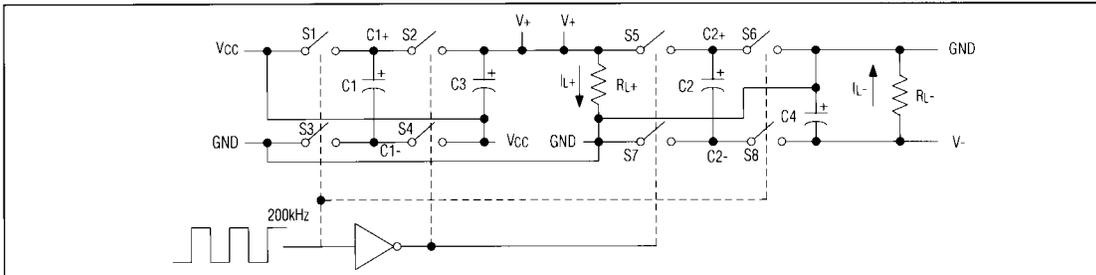
Figure 4. Dual Charge-Pump Diagram
