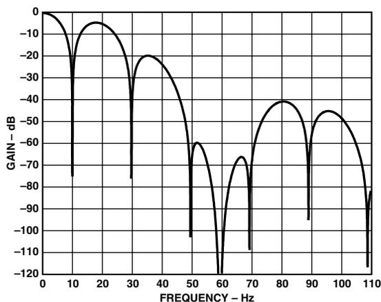
Figure 21. Filter Response, SF = 69 dec
