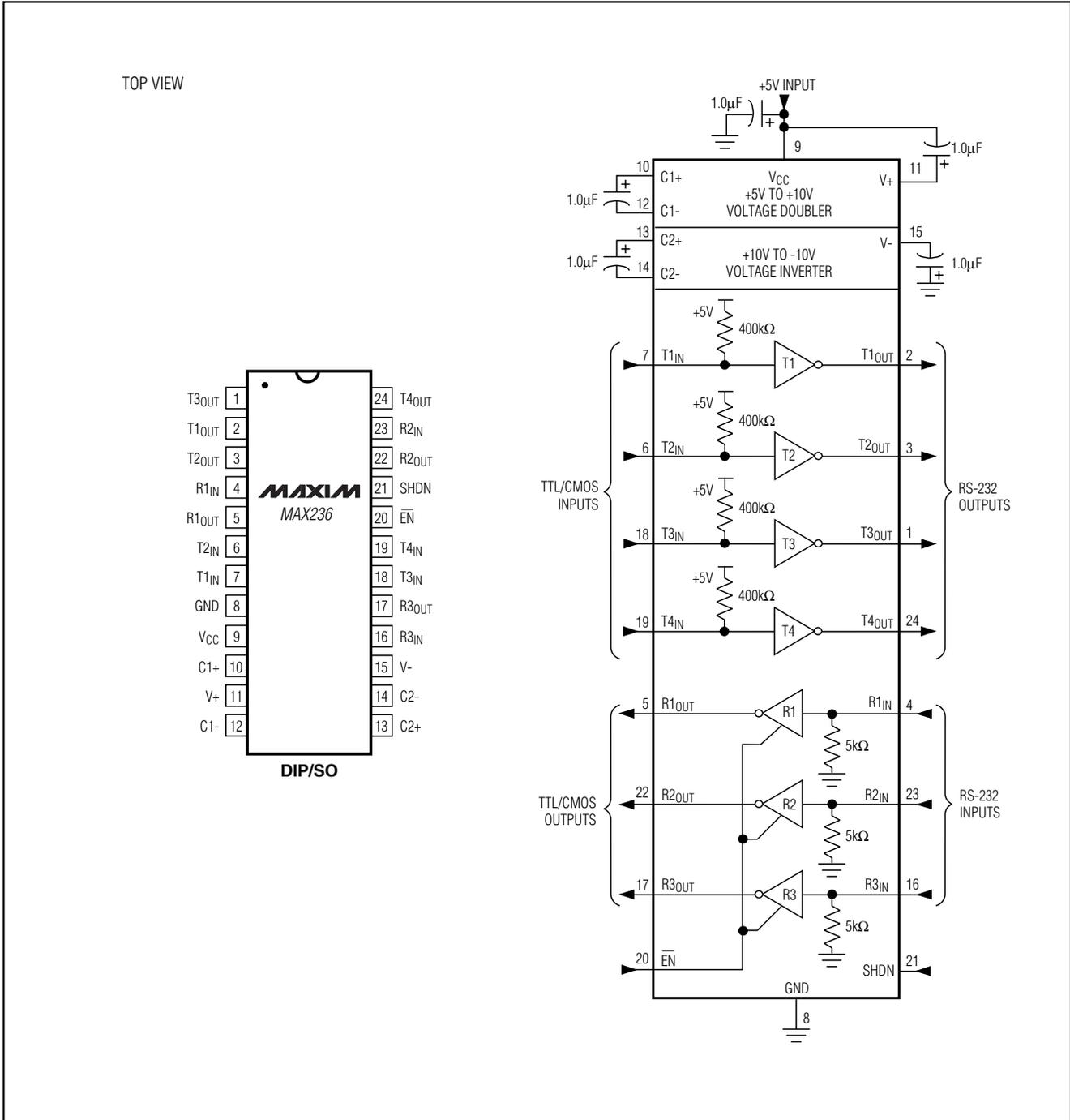
Figure 14. MAX236 Pin Configuration and Typical Operating Circuit
