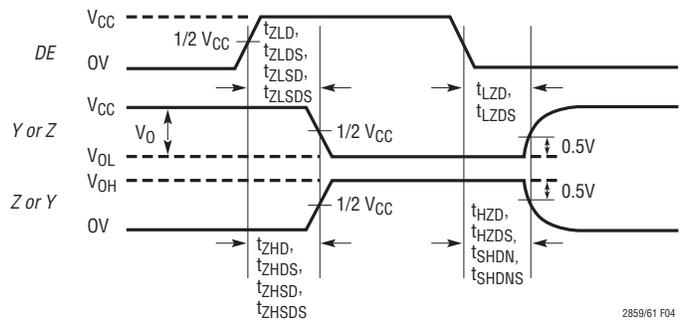
Figure 4. Driver Enable and Disable Timing Measurement
