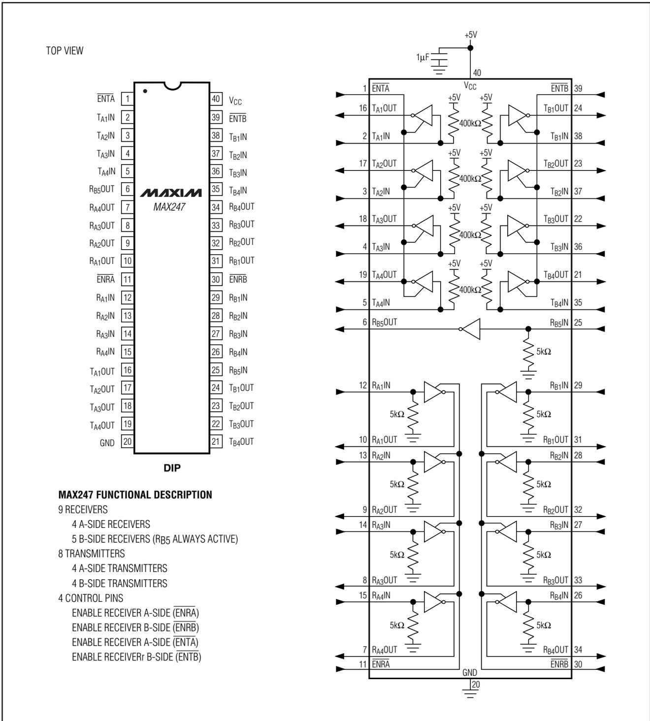
Figure 23. MAX247 Pin Configuration and Typical Operating Circuit
