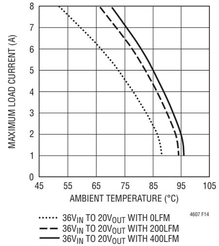
Figure 14. 36V<sub>IN</sub> to 20V<sub>OUT</sub> with Heat Sink
