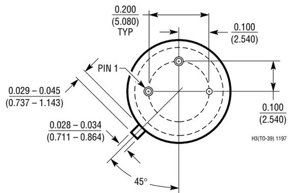
\* LEAD DIAMETER IS UNCONTROLLED BETWEEN THE REFERENCE PLANE AND 0.045" BELOW THE REFERENCE PLANE
