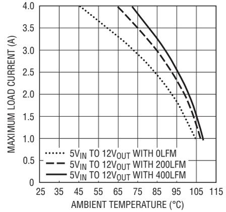
Figure 8. 5V<sub>IN</sub> to 12V<sub>OUT</sub> with Heatsink
