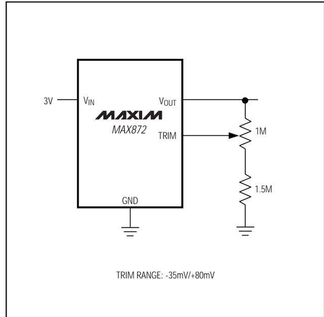
Figure 1a. Adjusting V<sub>OUT</sub> with the TRIM Input on the MAX872
