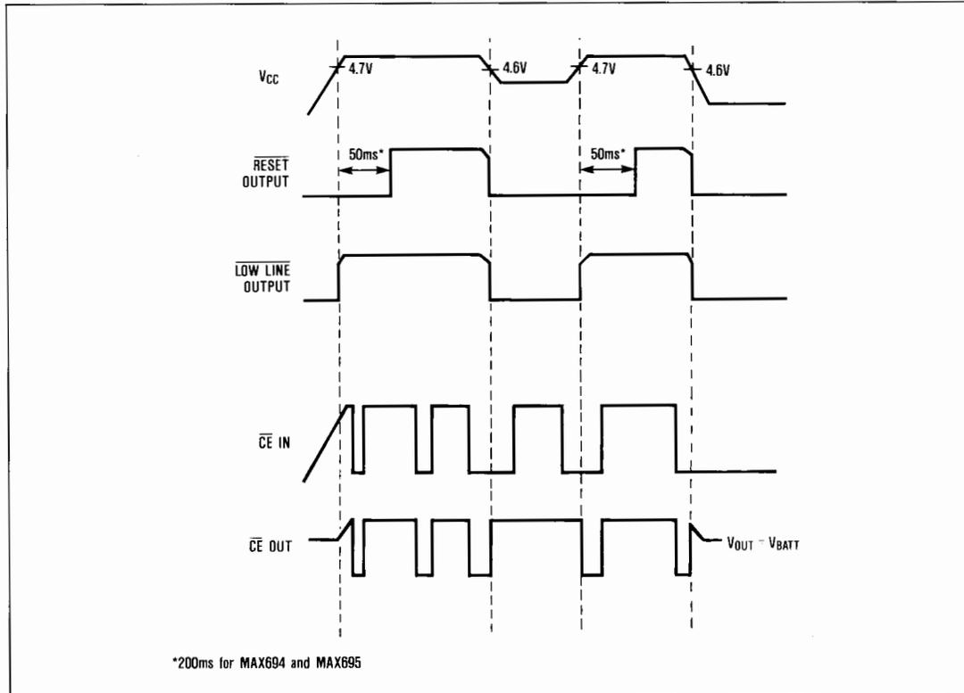
Figure 6. Reset Timing
