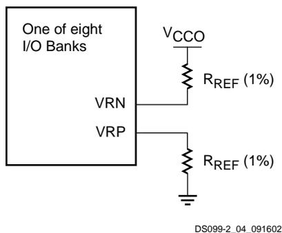
**Figure 3: Connection of Reference Resistors ( $R_{REF}$ )**
