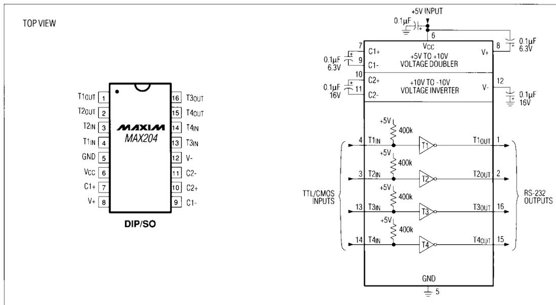
Figure 10. MAX204 Pin Configuration and Typical Operating Circuit
