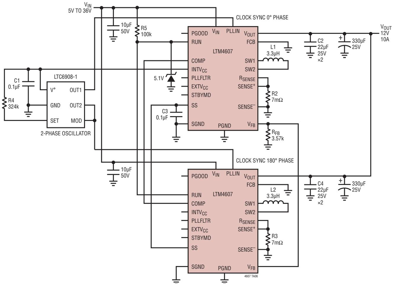
Figure 20. Two-Phase Parallel, 12V at 10A Design
