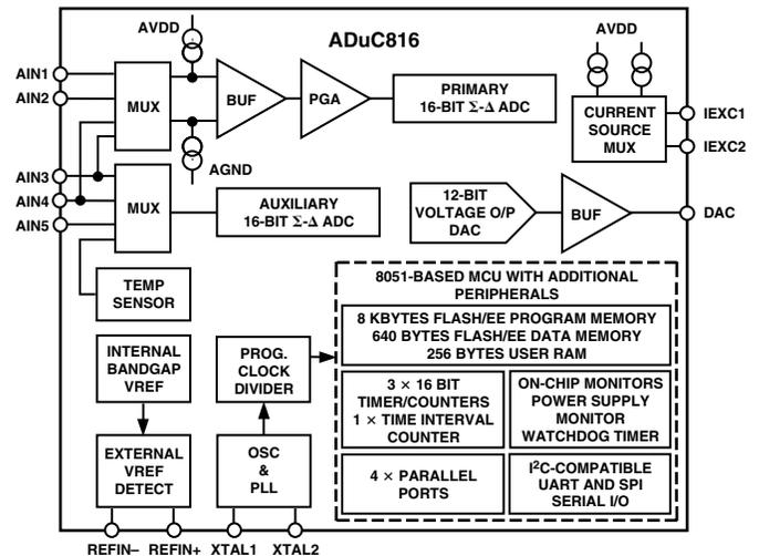
intended for the measurement of wide dynamic range, low frequency signals, such as those in weigh scale, strain gauge, pressure transducer, or temperature measurement applications. The ADC output data rates are programmable and the ADC output resolution will vary with the programmed gain and output rate.
