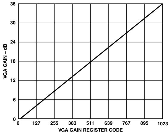
Figure 41. VGA Gain Curve (PxGA not included)
