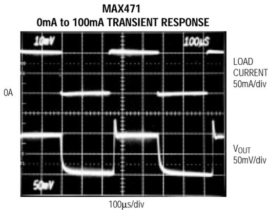
$V_{CC} = 10\text{V}$ ,  $R_{OUT} = 2k\Omega$  1%, SIGN PULL-UP =  $50k\Omega$  1%
