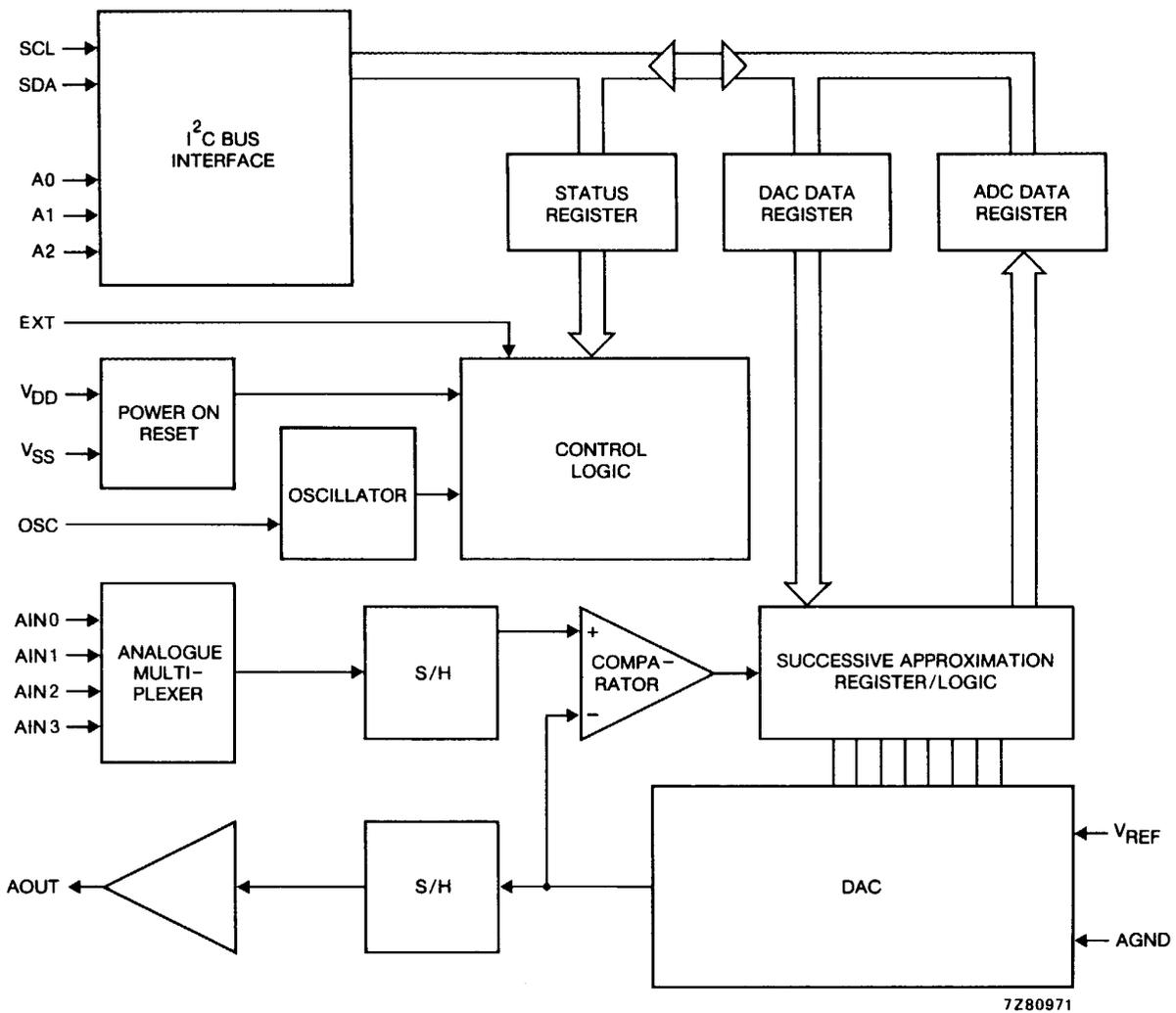
Fig.1 Block diagram.
