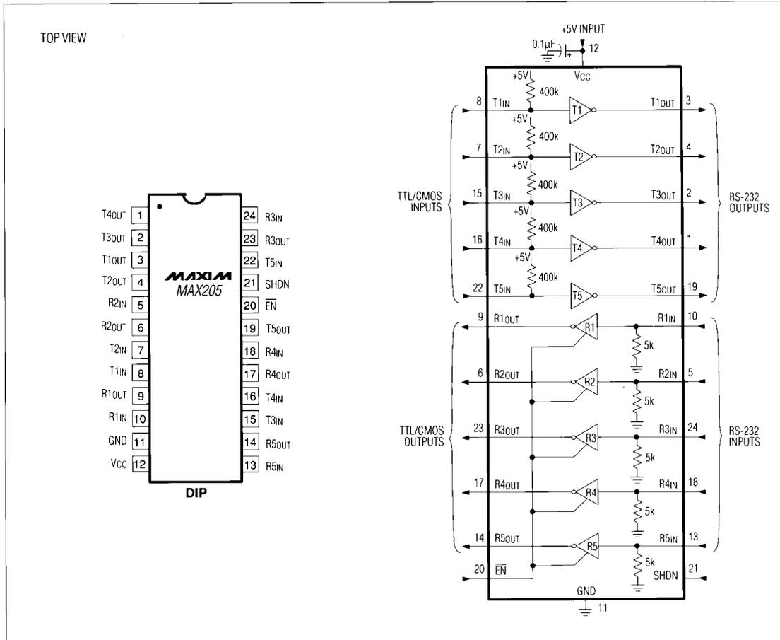
Figure 11. MAX205 Pin Configuration and Typical Operating Circuit
