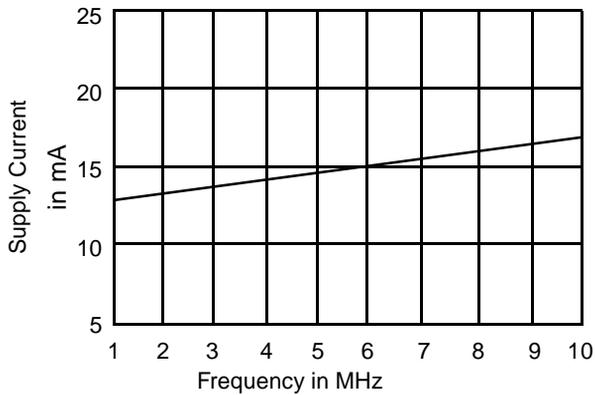
**Figure 1. Typical Supply Current vs. Frequency**
