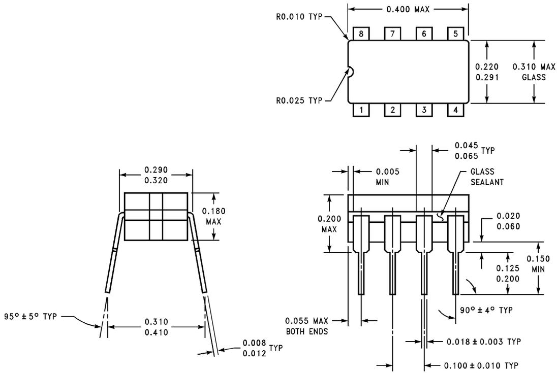
**8-Pin Ceramic Dual-In-Line Package**
