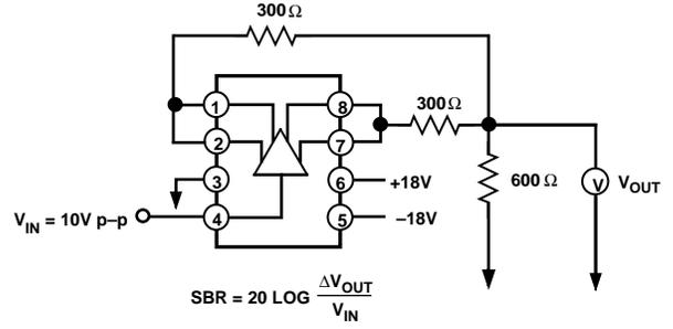
Figure 2. Signal Balance Ratio (BBC Method) Test Circuit
