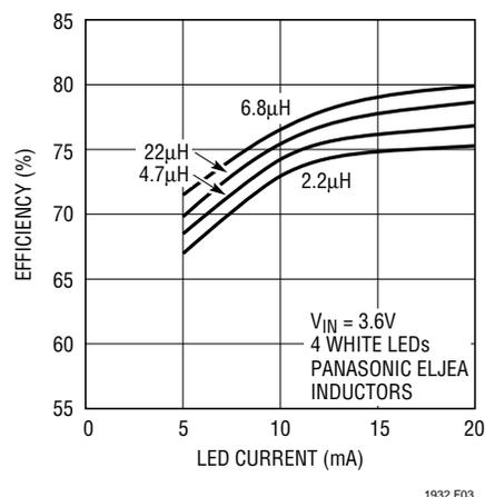
**Figure 3. Efficiency for Several Different Inductor Values**
