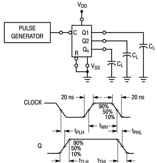
Figure 2. Switching Time Test Circuit and Waveforms
