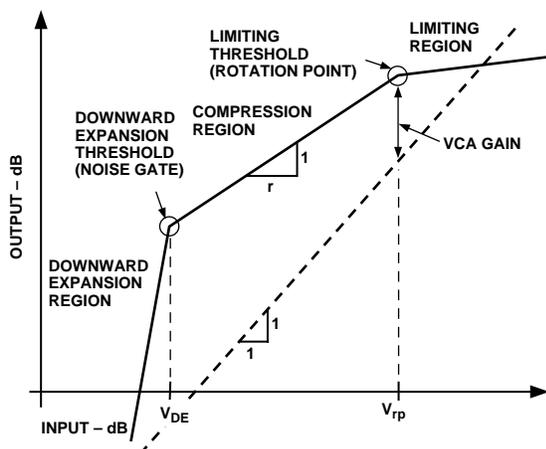
Figure 2. General Input/Output Characteristics of the SSM2165
