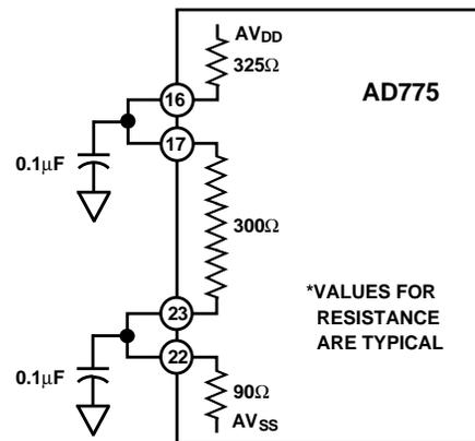
Figure 8. Reference Configuration: 0.64 V to 2.73 V
