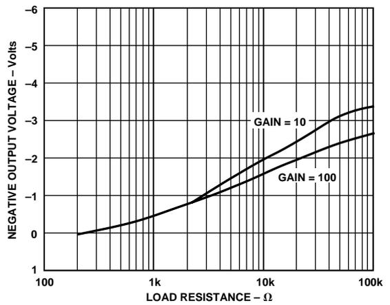
Figure 5. Negative Output Voltage Swing vs. Resistive Load
