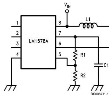
FIGURE 4. Current Limit Transient Suppressor, Ground Referred
