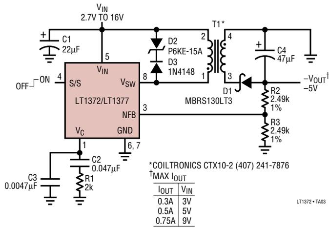
Dual Output Flyback Converter with Overvoltage Protection
