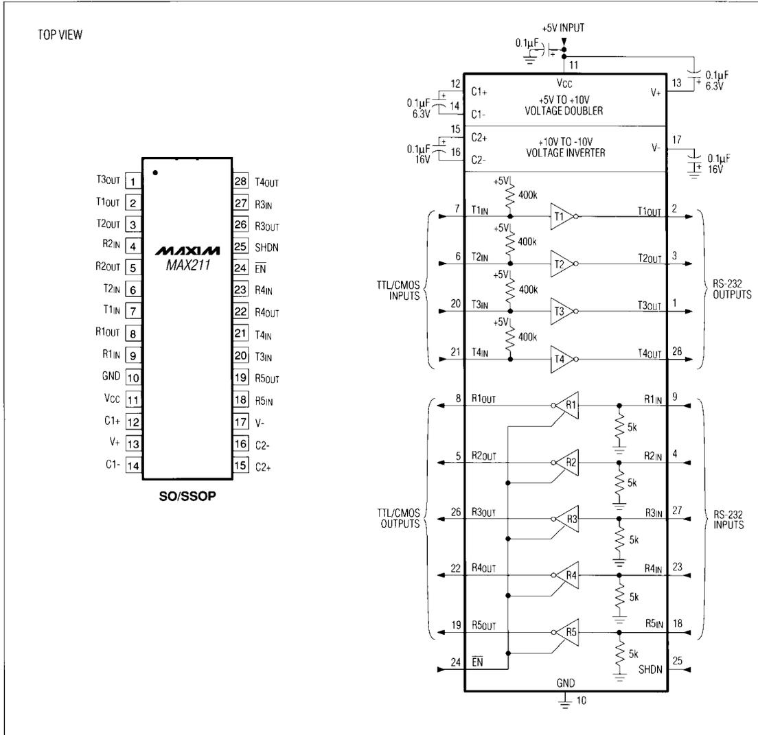
Figure 16. MAX211 Pin Configuration and Typical Operating Circuit
