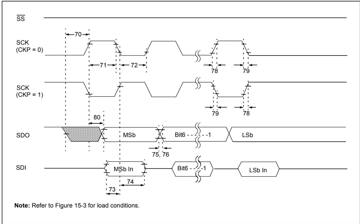
**FIGURE 15-11: SPI MASTER MODE TIMING (CKE = 1, SMP = 1)**
