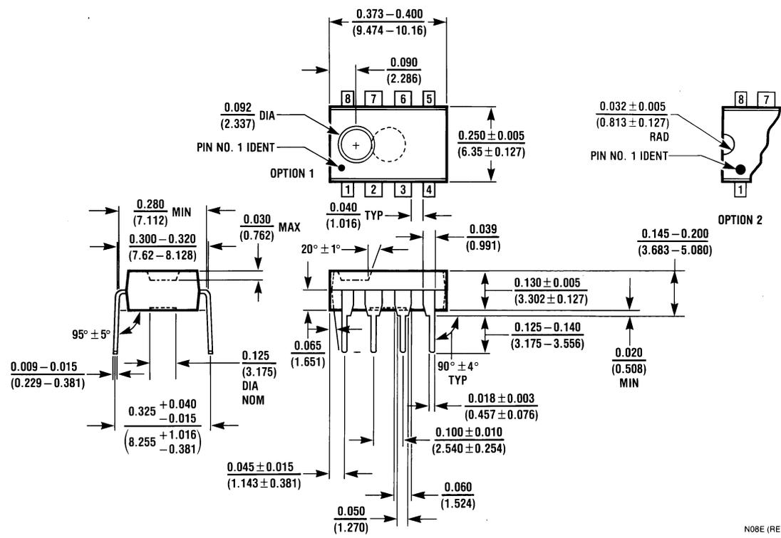
**8-Pin Molded Dual-In-Line Package**
