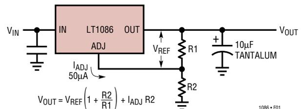
Figure 1. Basic Adjustable Regulator
