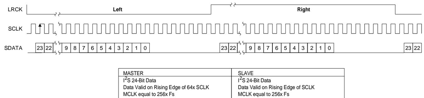
**Figure 3. Serial Data Format 1, Stand-Alone Mode, DFS High. I<sup>2</sup>S compatible**
