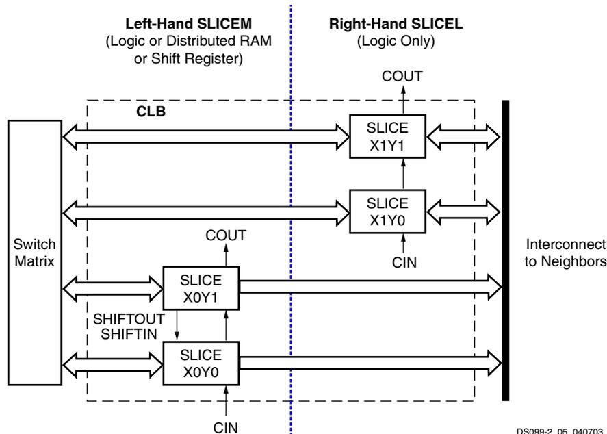
Figure 5: Arrangement of Slices within the CLB
