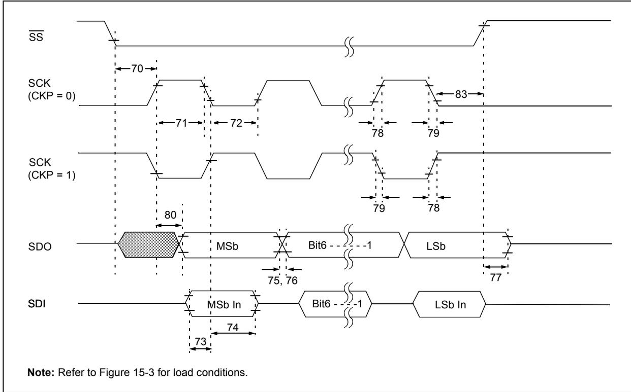
**FIGURE 15-13: SPI SLAVE MODE TIMING (CKE = 1)**
