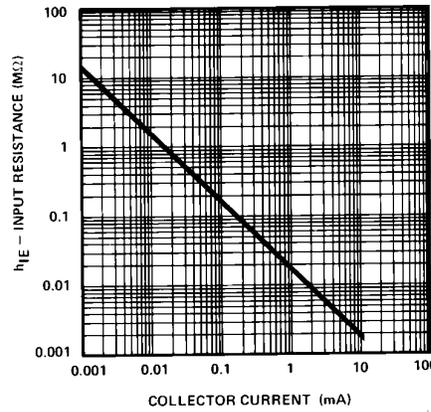
Figure 5. Small Signal Input Resistance vs. Collector Current
