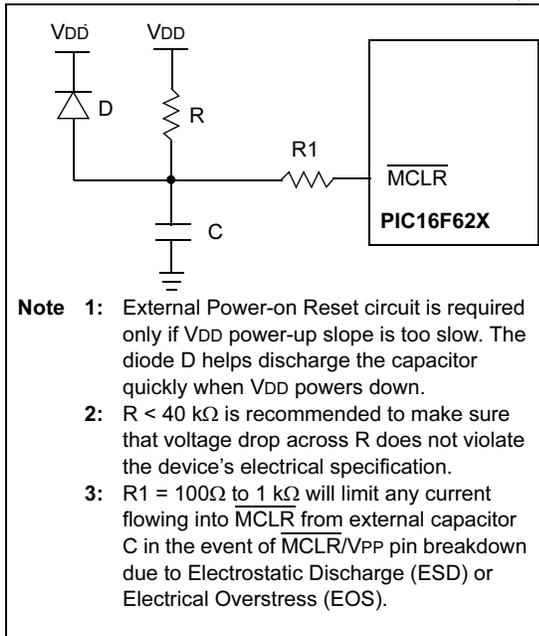
**FIGURE 14-13: EXTERNAL BROWN-OUT PROTECTION CIRCUIT 2**
