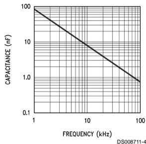
FIGURE 1. Value of Timing Capacitor vs Oscillator Frequency
