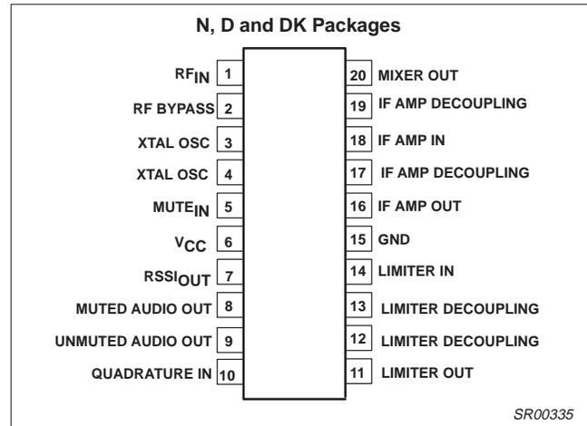
Figure 1. Pin Configuration
