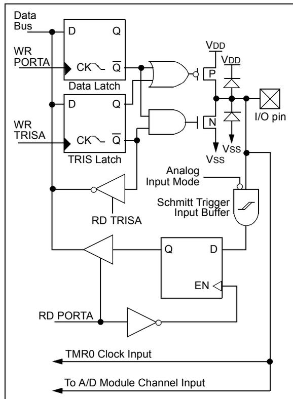
**FIGURE 5-5: BLOCK DIAGRAM OF RA5/MCLR/VPP PIN**
