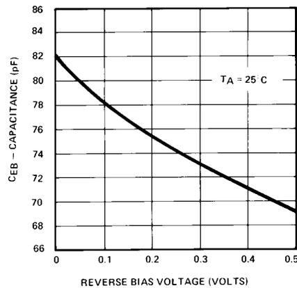
Figure 17. Emitter-Base Capacitance vs. Reverse Bias Voltage
