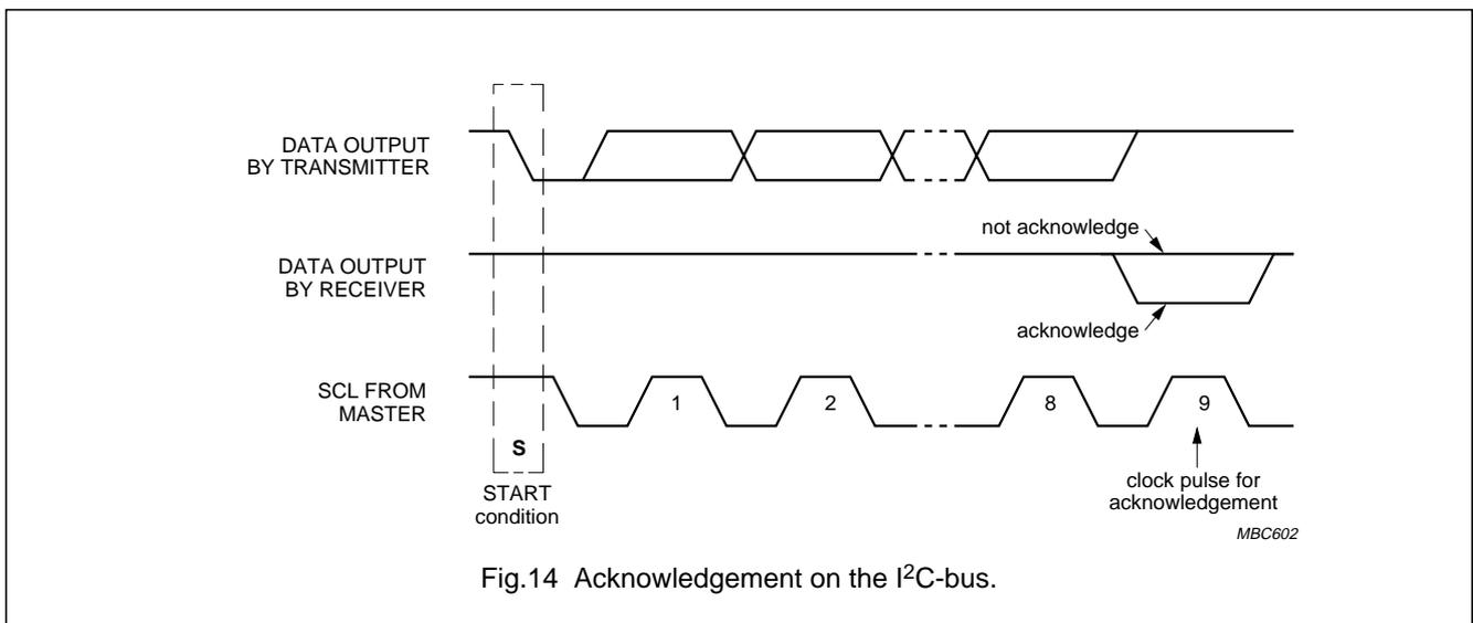
Fig.14 Acknowledgement on the I<sup>2</sup>C-bus.
