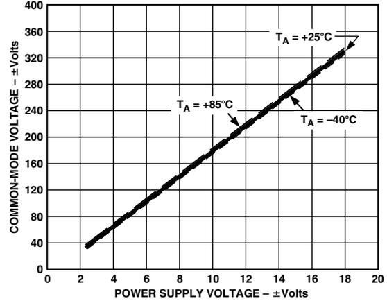
Figure 8. Common-Mode Operating Range vs. Power Supply Voltage
