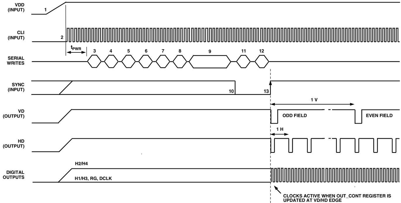
Figure 42. Recommended Power-Up Sequence and Synchronization, Master Mode
