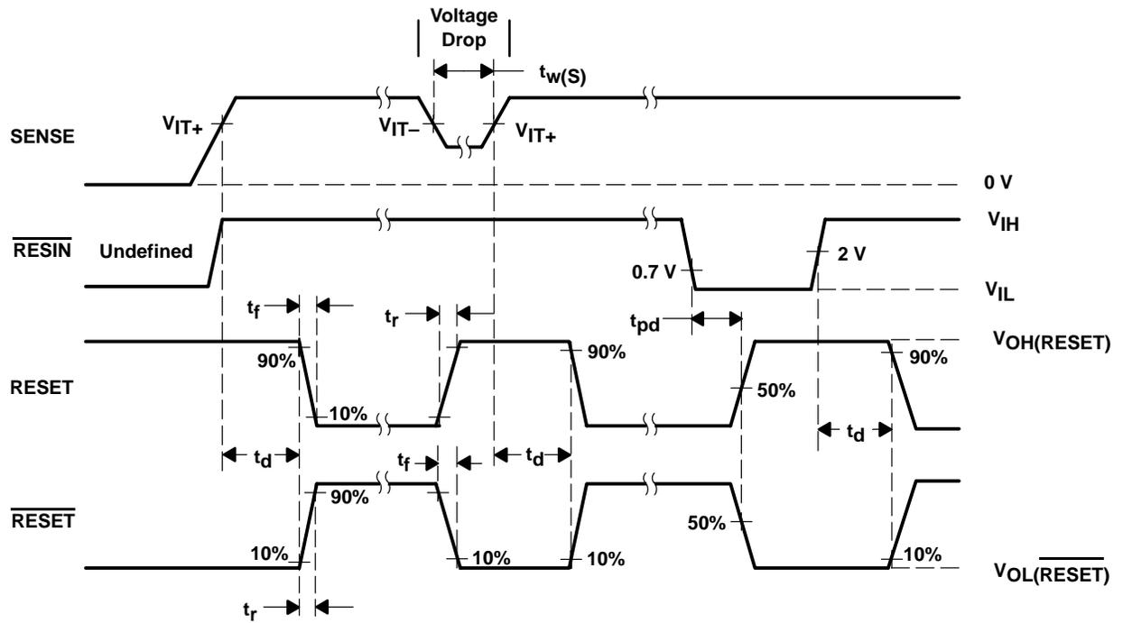
Figure 1. Voltage Waveforms
