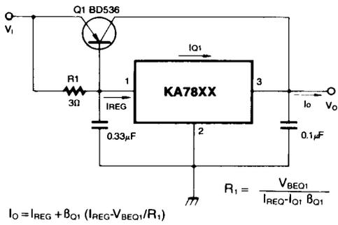
Fig. 13 High Output Current with Short Circuit Protection
