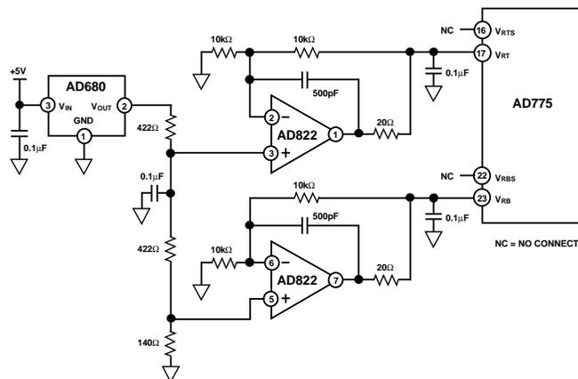
Figure 11. Reference Configuration: 0.7 V to 3.2 V
