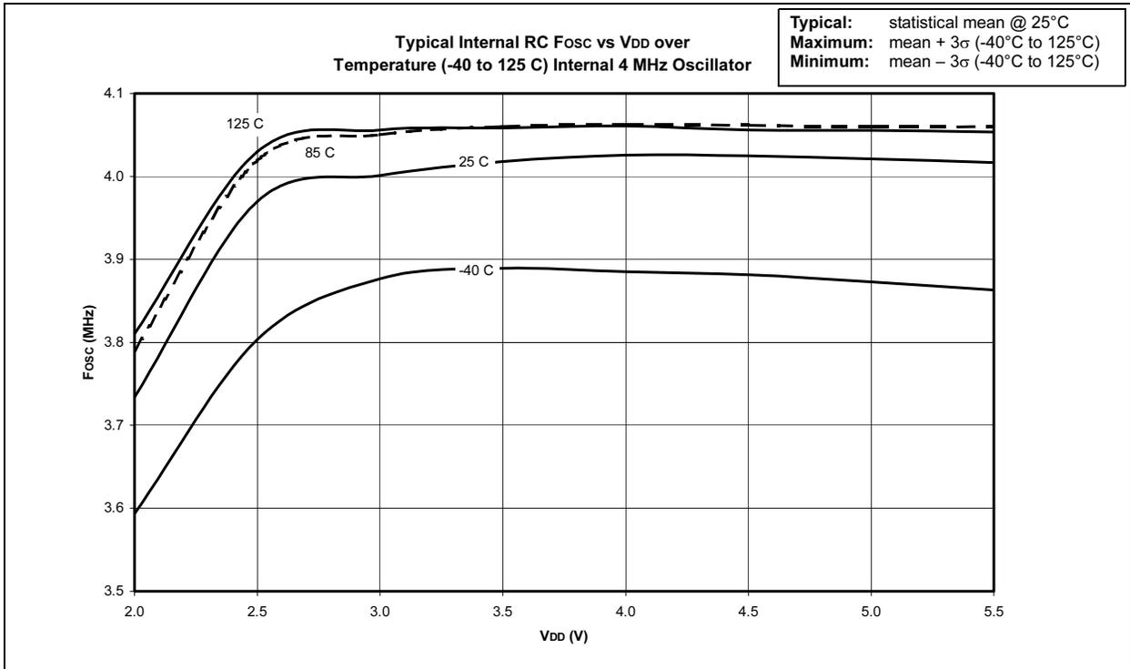
**FIGURE 18-9: TYPICAL INTERNAL RC Fosc vs VDD OVER TEMPERATURE (-40 TO 125°C)
