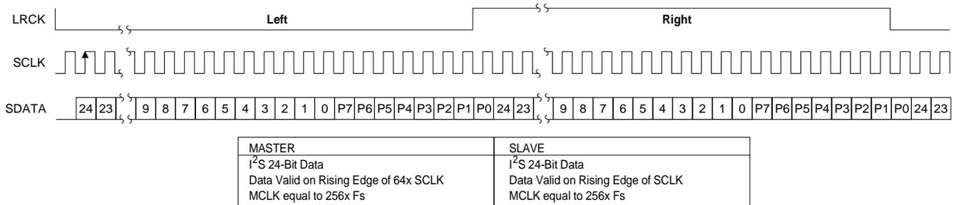
**Figure 5. Control Port Mode, Serial Data. I<sup>2</sup>S Compatible. 64x Oversampling Mode.**
