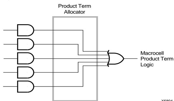
Figure 5: Macrocell Logic Using Direct Product Term
