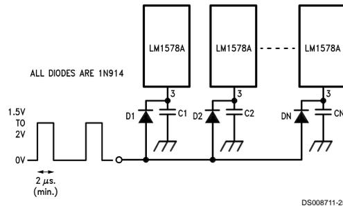
FIGURE 13. Synchronizing Devices
