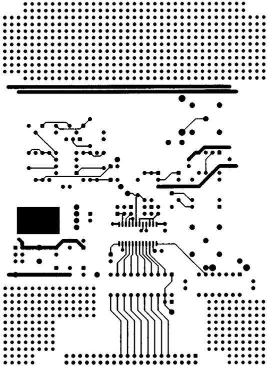
Figure 19. Component Side PCB Layout (Not to Scale)
