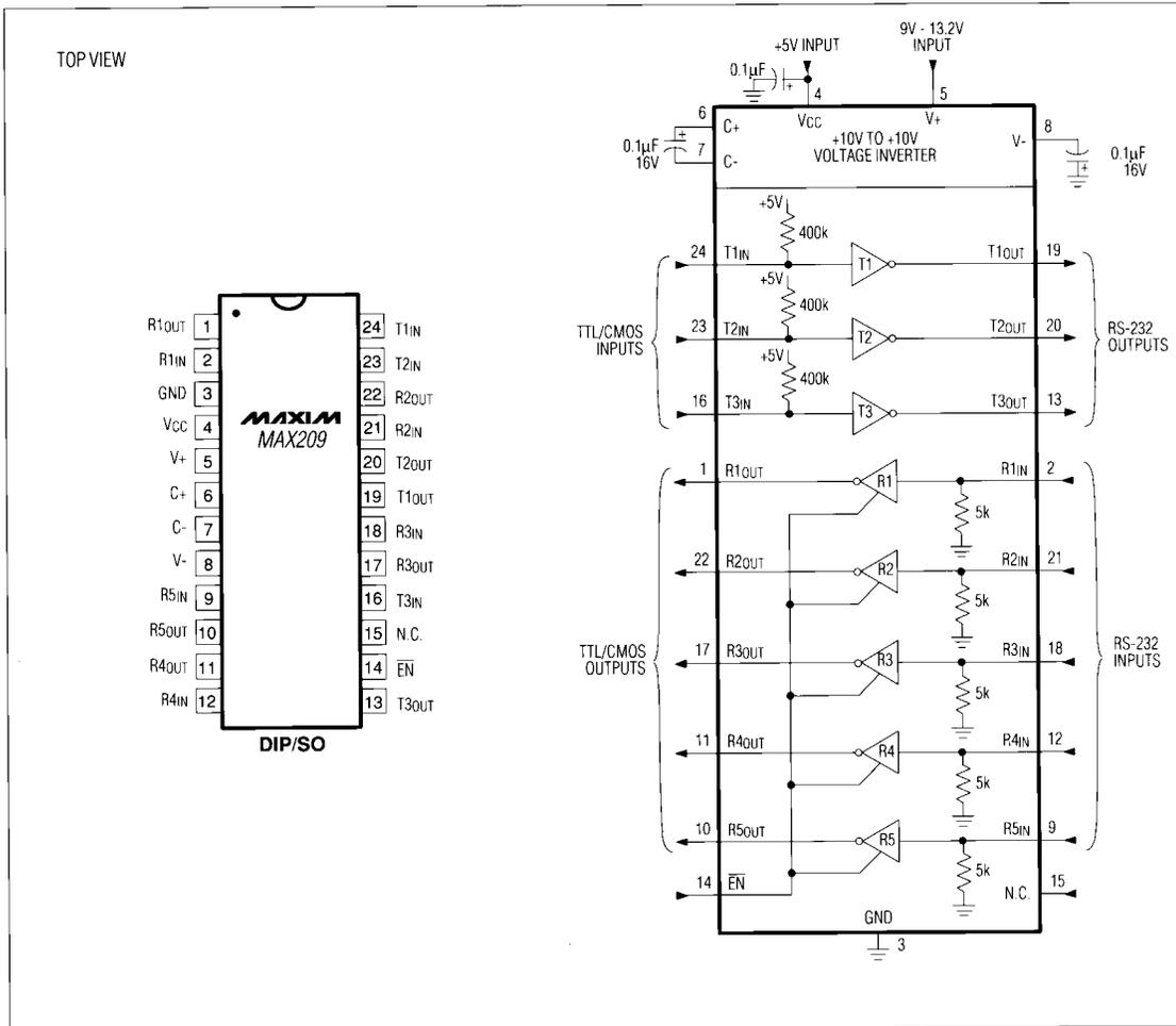
Figure 15. MAX209 Pin Configuration and Typical Operating Circuit
