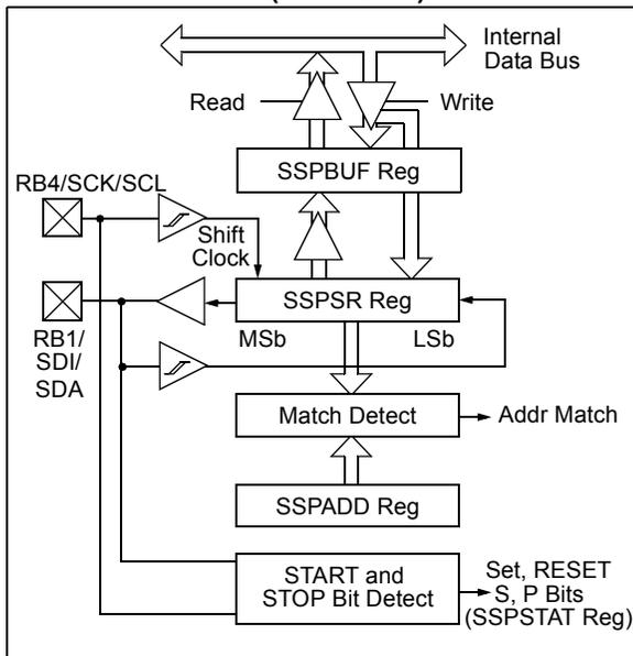
The SSP module has five registers for I<sup>2</sup>C operation:
