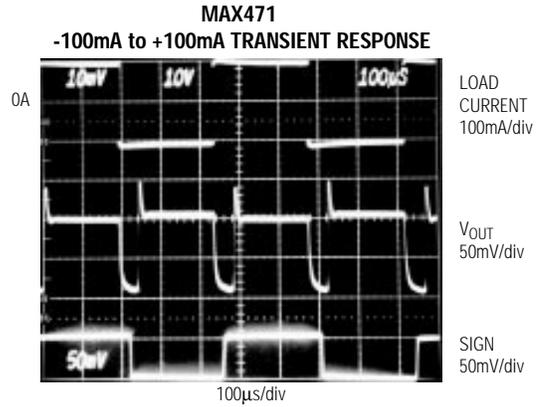
$V_{CC} = 10\text{V}$ ,  $R_{OUT} = 2k\Omega$  1%, SIGN PULL-UP =  $50k\Omega$  1%
