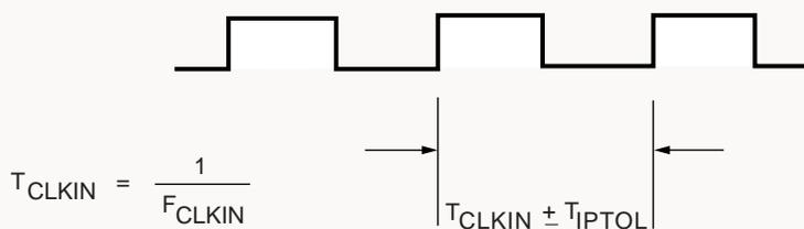
**Output Jitter:** the difference between an ideal reference clock edge and the actual design.
