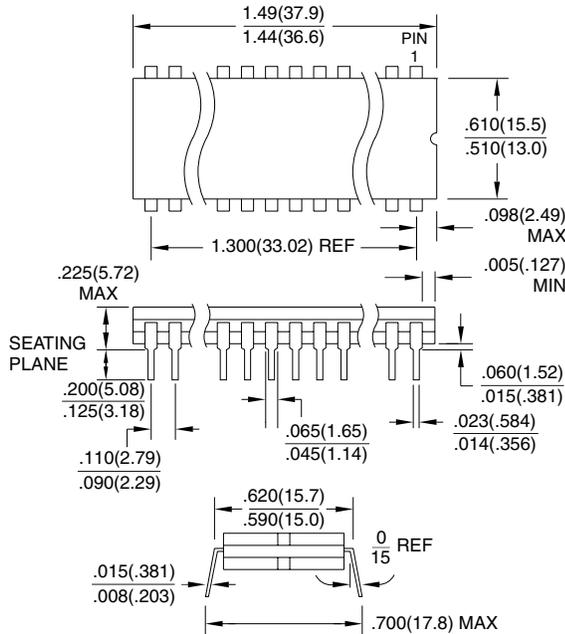
**28F**, 28-lead, Non-windowed, Ceramic Bottom-brazed Flat Package (Flatpack)
