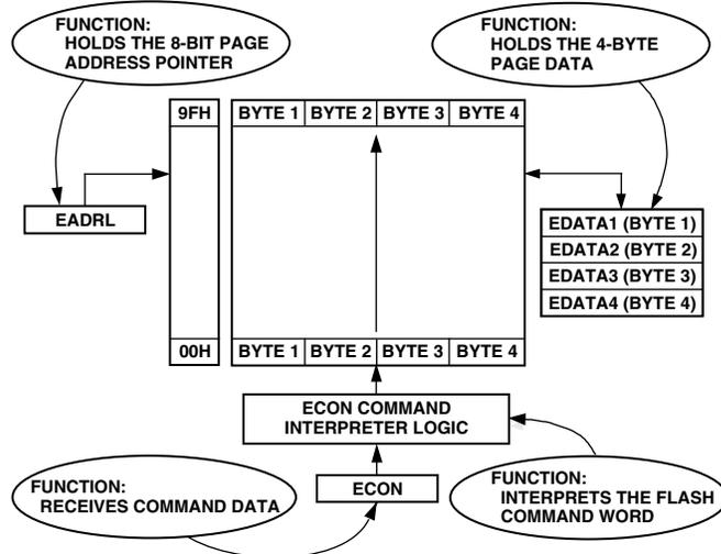
Figure 30. Flash/EE Data Memory Control and Configuration
