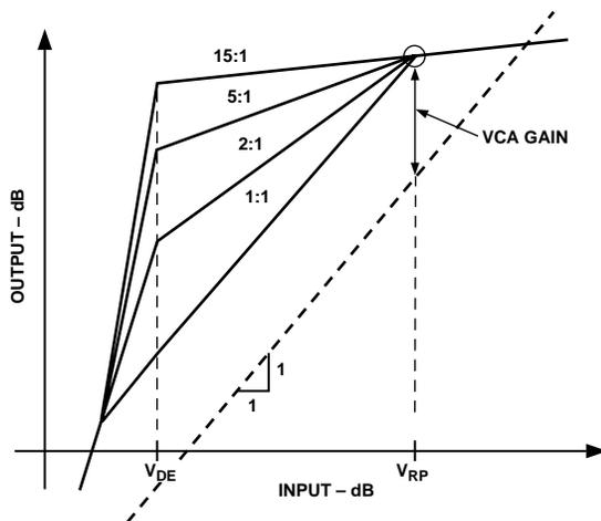
Figure 6. Effect of Varying the Compression Ratio
