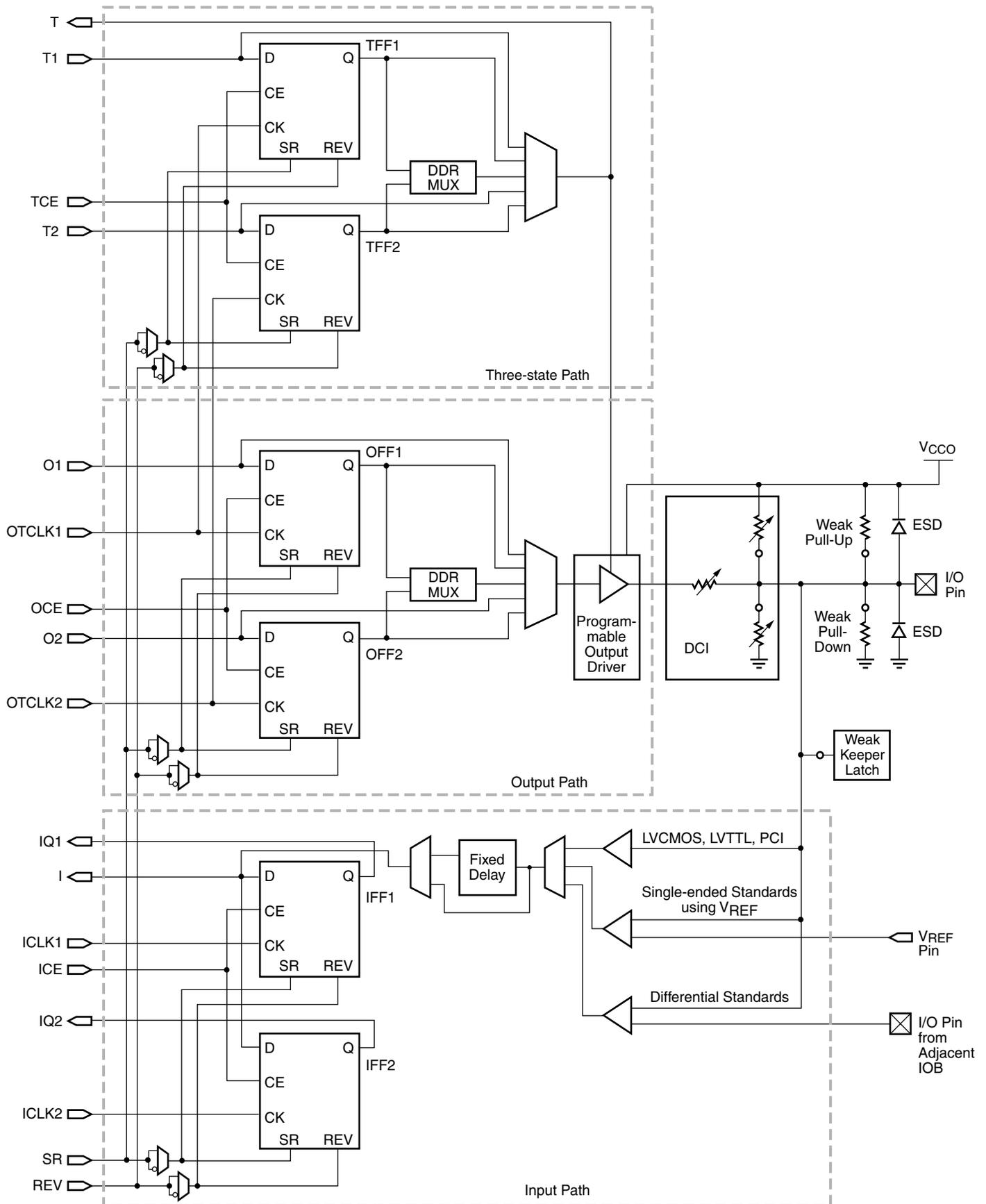
Note: All IOB signals communicating with the FPGA's internal logic have the option of inverting polarity.
