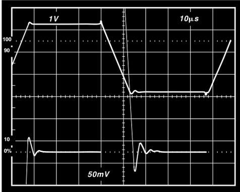
Figure 25. Settling Time.  $V_S = +5\text{ V}$ ,  $G = 10$
