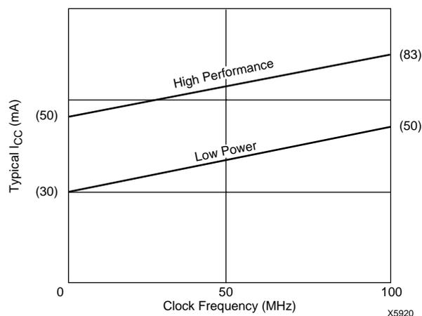
**Figure 1: Typical I<sub>CC</sub> vs. Frequency For XC9536**
