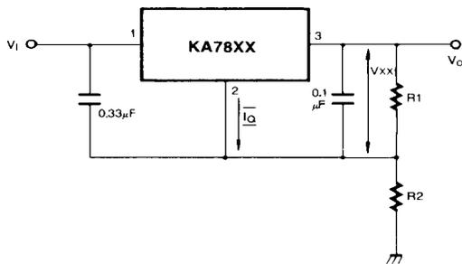
Fig. 11 Adjustable Output Regulator (7 to 30V)
