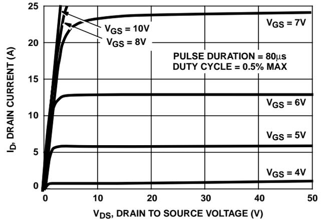
FIGURE 5. OUTPUT CHARACTERISTICS
