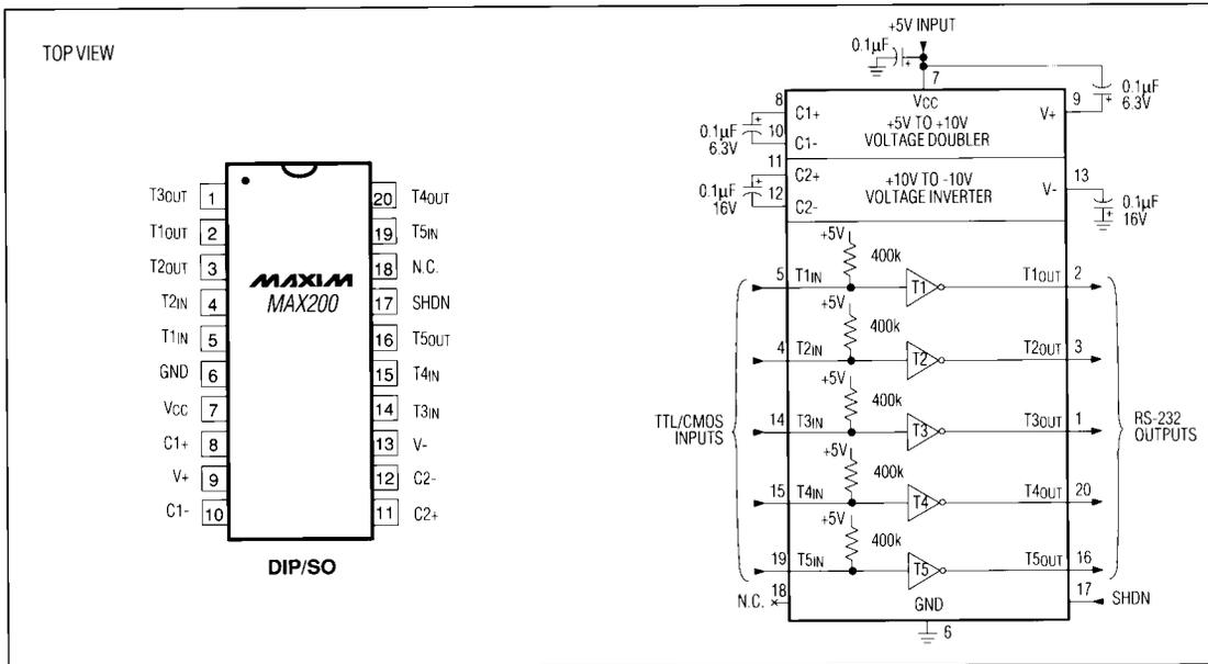
Figure 6. MAX200 Pin Configuration and Typical Operating Circuit
