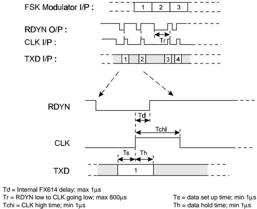
**Figure 6c FSK Operation with Tx Data Retiming**
