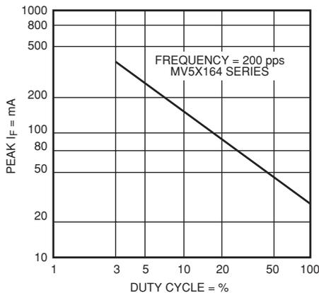
**Fig. 3. Max Peak Current vs. Duty Cycle**
