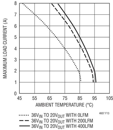
Figure 13. 36V<sub>IN</sub> to 20V<sub>OUT</sub> without Heat Sink
