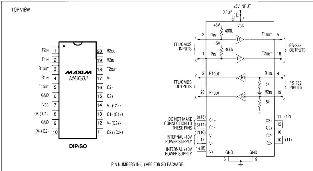
Figure 9. MAX203 Pin Configuration and Typical Operating Circuit
