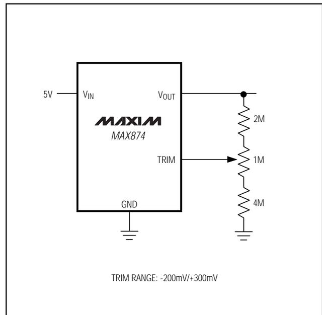
Figure 1b. Adjusting V<sub>OUT</sub> with the TRIM Input on the MAX874
