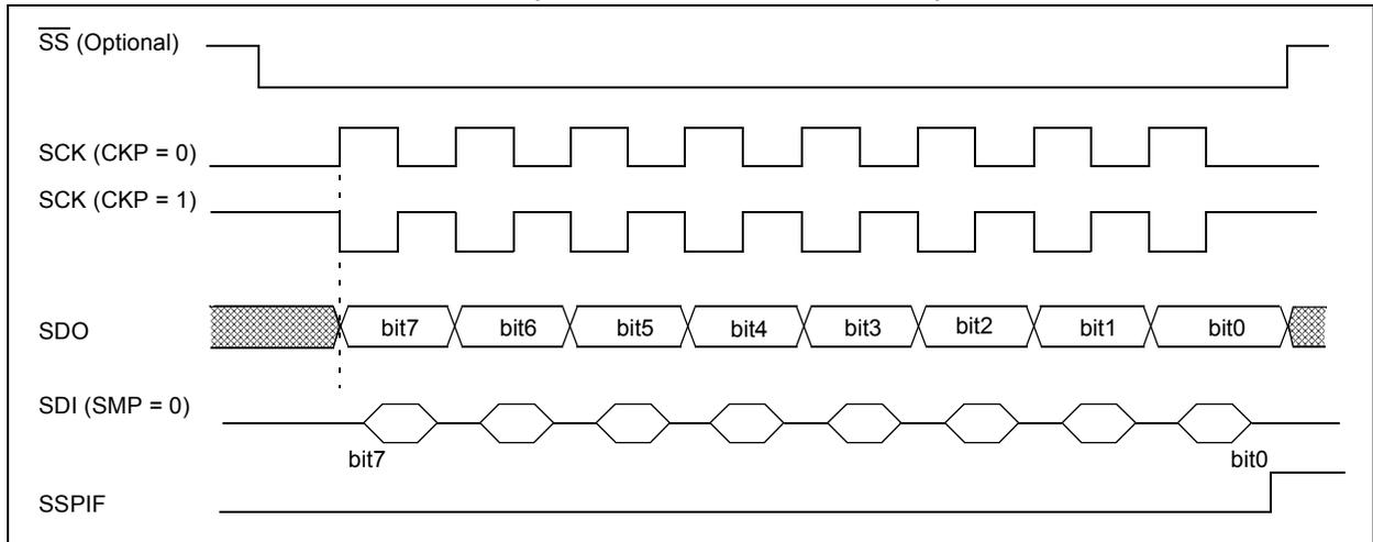
**FIGURE 10-4: SPI MODE TIMING (SLAVE MODE WITH CKE = 1)**
