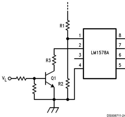
FIGURE 11. Shutdown Occurs when  $V_L$  is High
