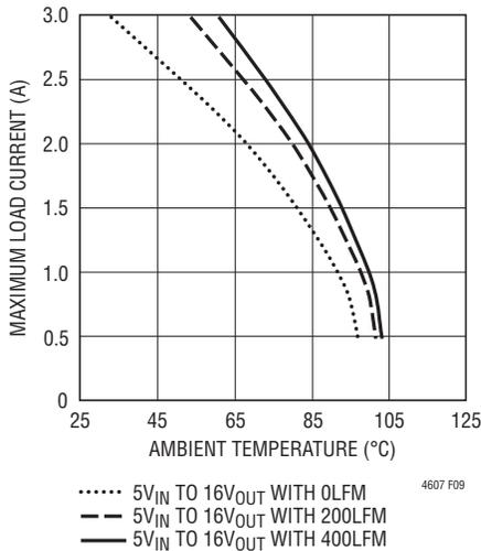
Figure 9. 5V<sub>IN</sub> to 16V<sub>OUT</sub> without Heatsink
