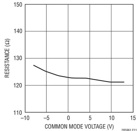
**Figure 11. Termination Resistance vs Common Mode Voltage**
