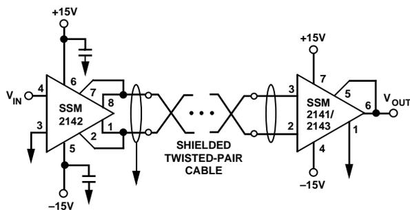
Figure 14. Typical Application of the SSM2142 and SSM2141
