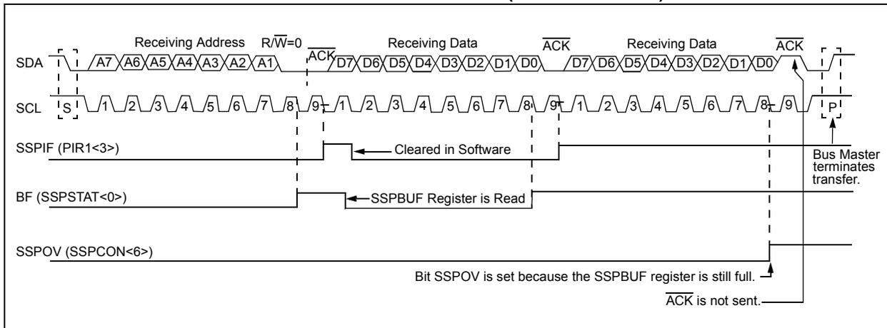
**FIGURE 10-7: I<sup>2</sup>C WAVEFORMS FOR TRANSMISSION (7-BIT ADDRESS)**
