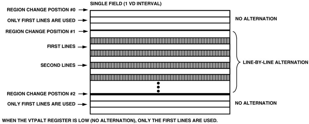
Figure 23. Use of Line Alteration in Vertical Sequencing
