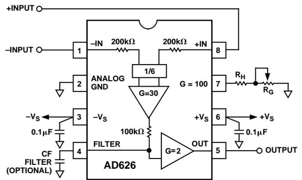
$$\text{CORNER FREQUENCY OF FILTER} = \frac{1}{2\pi CF (100k\Omega)}$$
