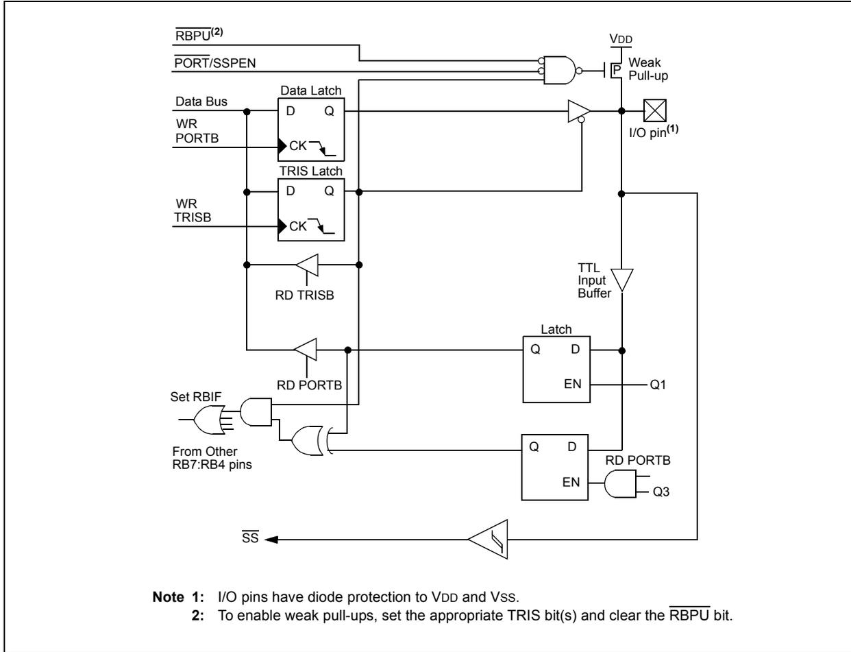
**FIGURE 5-14: BLOCK DIAGRAM OF RB6 PIN**
