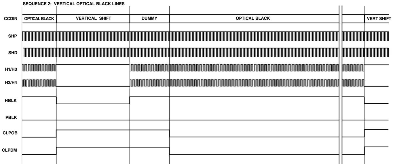
Figure 47. Horizontal Sequences During Vertical Optical Black Pixels
