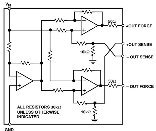
Based on a cross-coupled, electronically balanced topology, the SSM2142 mimics the performance of fully balanced transformer-based solutions for line driving. However, the SSM2142 maintains lower distortion and occupies much less board space than transformers while achieving comparable common-mode rejection performance with reduced parts count.
