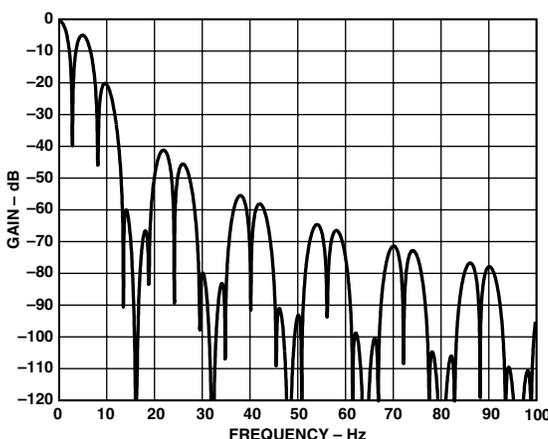
Figure 22. Filter Response, SF = 255 dec
