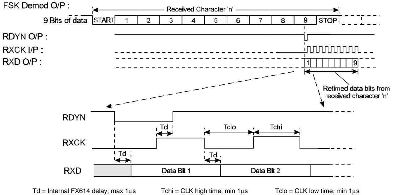
**Figure 6a FSK Operation with Rx Data Retiming**
