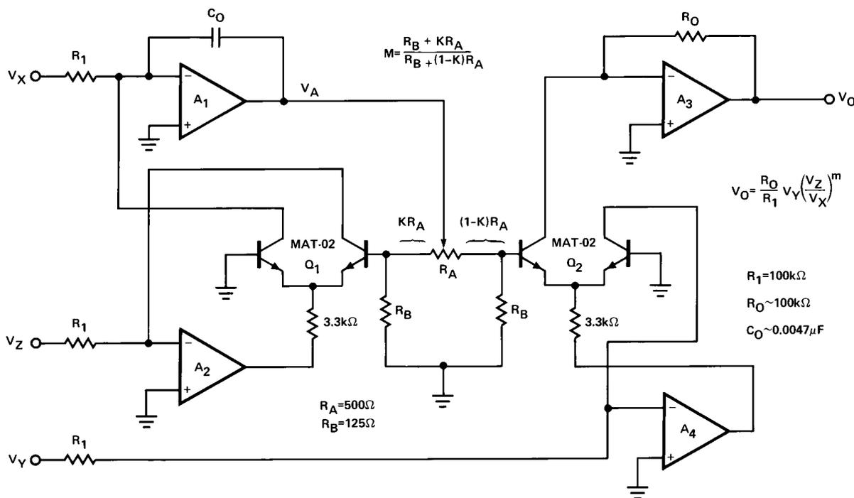
Figure 22. Multifunction Converter
