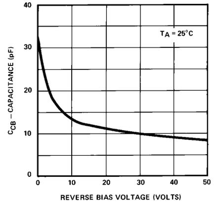
Figure 15. Collector-Base Capacitance vs. Reverse Bias Voltage
