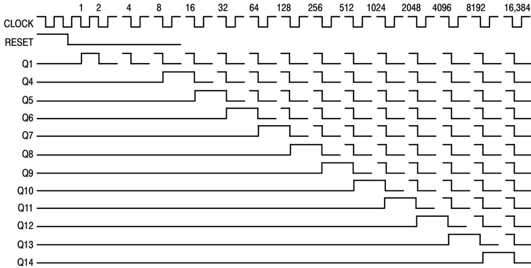
**Figure 3. Timing Diagram**
