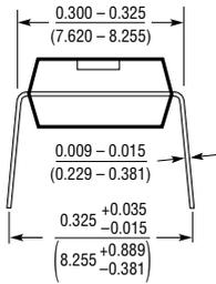
\*THESE DIMENSIONS DO NOT INCLUDE MOLD FLASH OR PROTRUSIONS.
