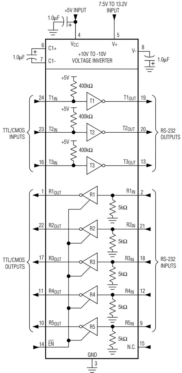
Figure 17. MAX239 Pin Configuration and Typical Operating Circuit
