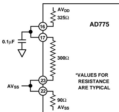
Figure 9. Reference Configuration: 0 V to +2.4 V
