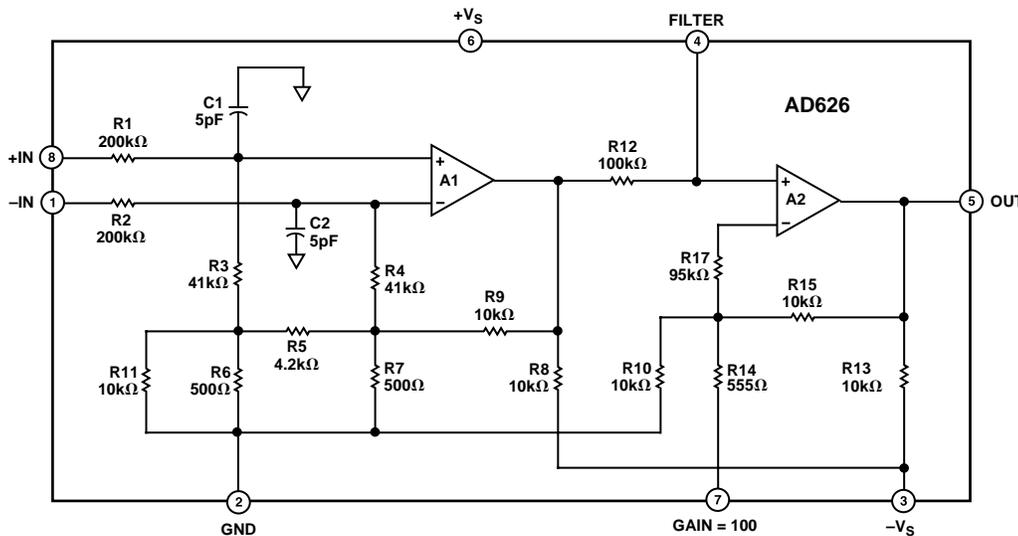
Figure 28. Simplified Schematic
