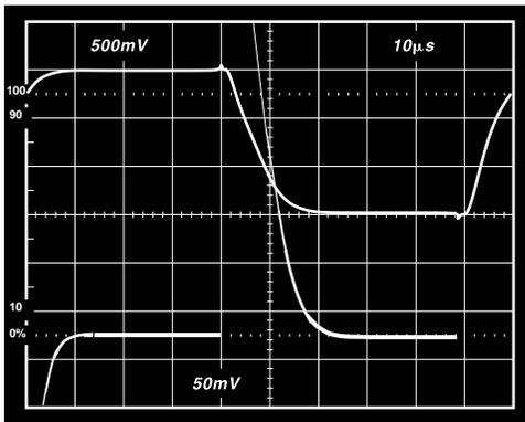
Figure 26. Settling Time.  $V_S = +5\text{ V}$ ,  $G = 100$
