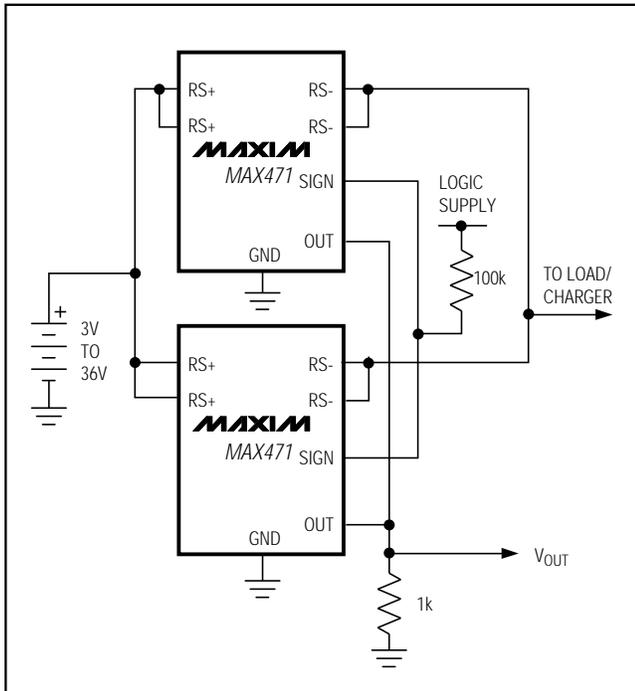
Figure 3. Paralleling MAX471s to Sense Higher Load Current
