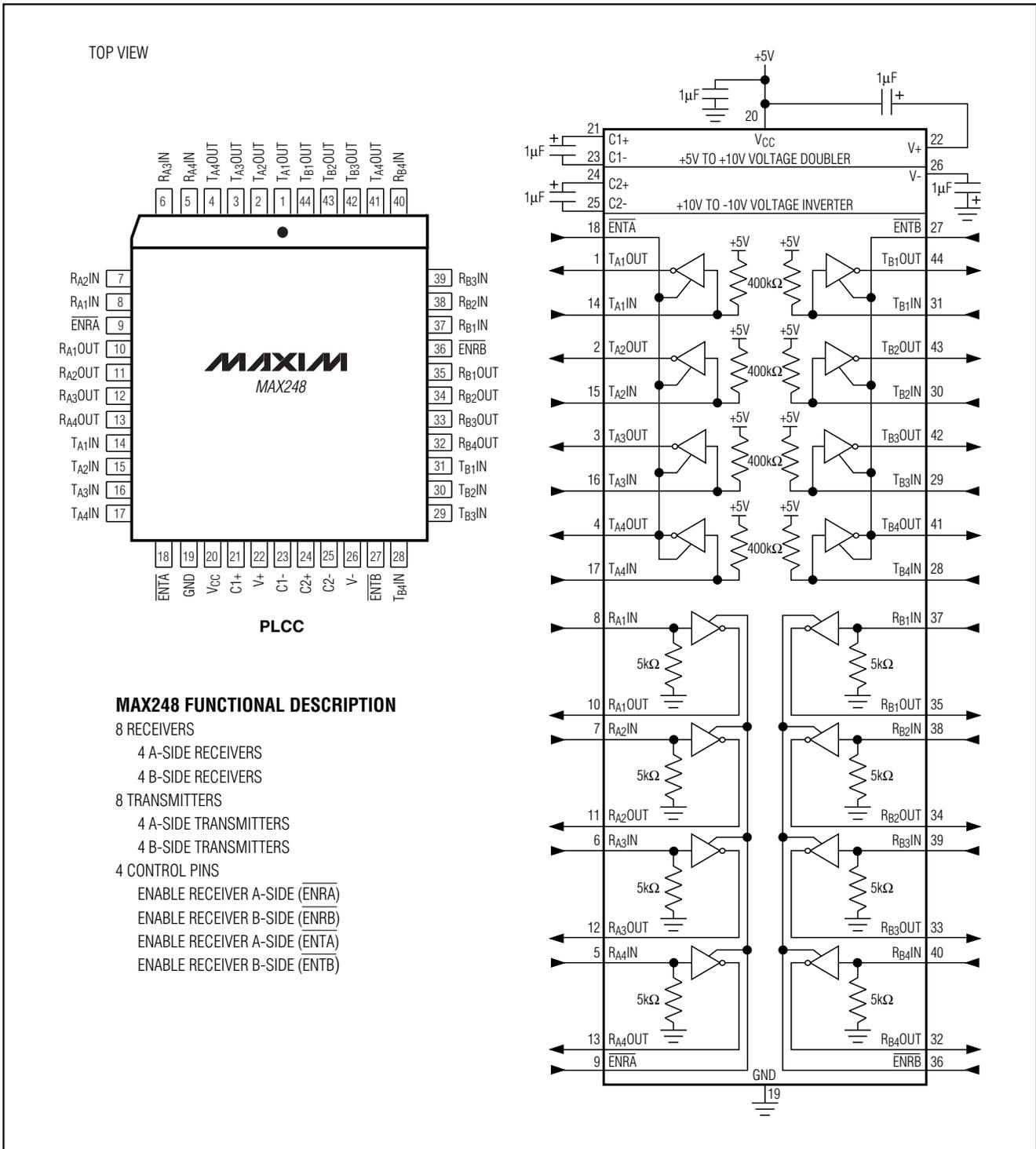
Figure 24. MAX248 Pin Configuration and Typical Operating Circuit
