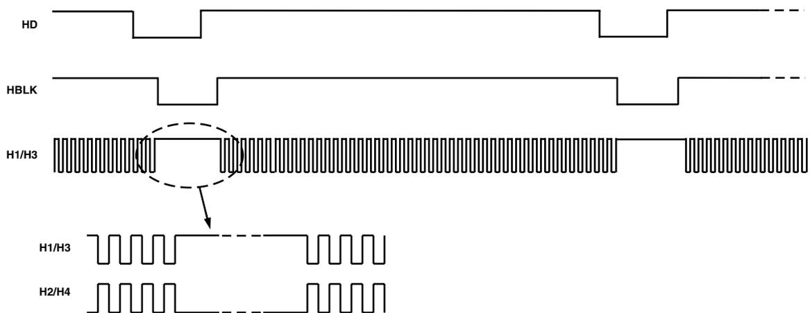
THE POLARITY OF H1 DURING BLANKING IS PROGRAMMABLE (H2 IS OPPOSITE POLARITY OF H1)
