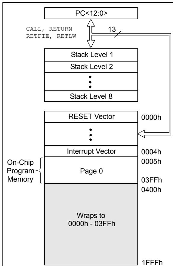
**FIGURE 2-2: PROGRAM MEMORY MAP AND STACK FOR PIC16F819**
