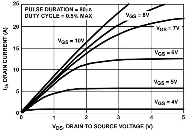
FIGURE 6. SATURATION CHARACTERISTICS
