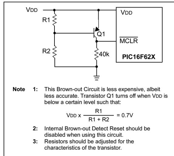
**FIGURE 14-12: EXTERNAL BROWN-OUT PROTECTION CIRCUIT 1**
