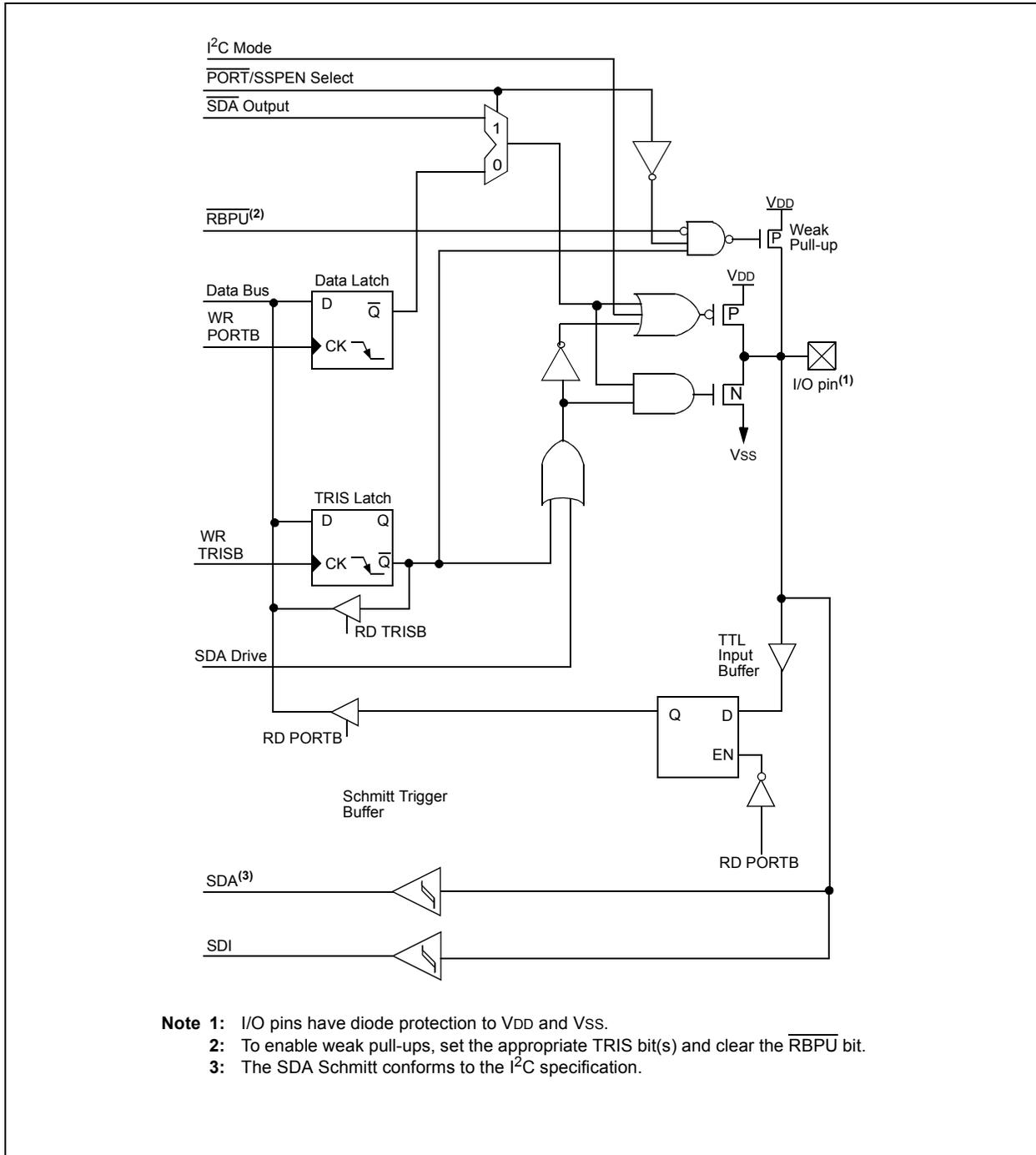
**FIGURE 5-10: BLOCK DIAGRAM OF RB2 PIN**
