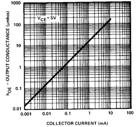
Figure 6. Small-Signal Output Conductance vs. Collector Current
