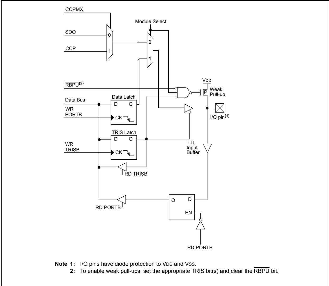
FIGURE 5-12: BLOCK DIAGRAM OF RB4 PIN
