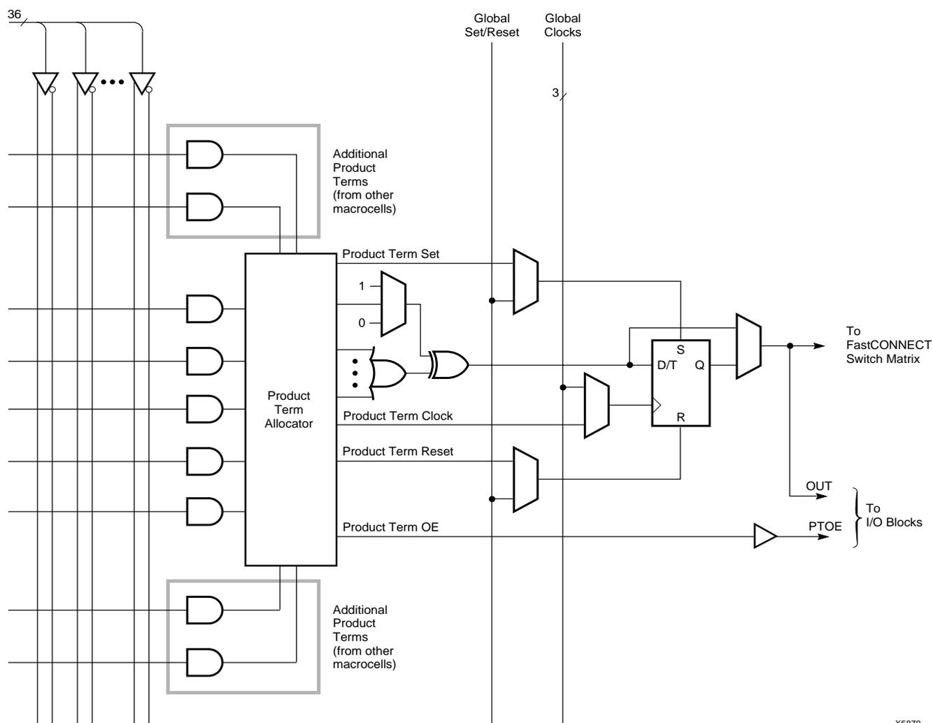
**Figure 3: XC9500 Macrocell Within Function Block**
