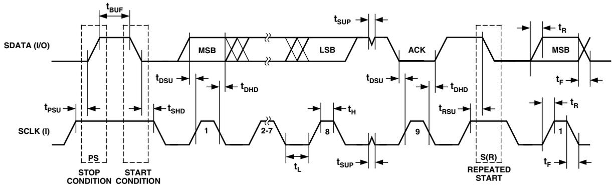
Figure 7. I<sup>2</sup>C-Compatible Interface Timing
