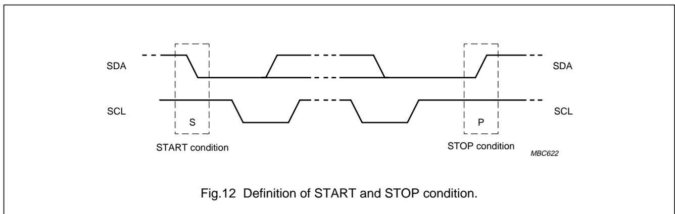
Fig.12 Definition of START and STOP condition.
