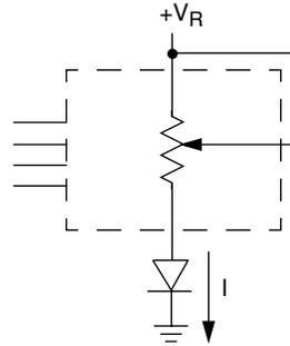
Two terminal Variable Resistor;
