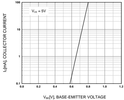
Figure 2. Transfer Characteristic
