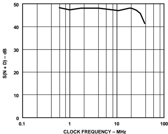
Figure 14.  $S/(N + D)$  vs. Clock Frequency (Temperature = +25°C)
