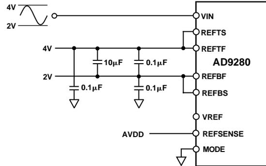
Figure 23a. External Reference—2 V p-p Input Span
