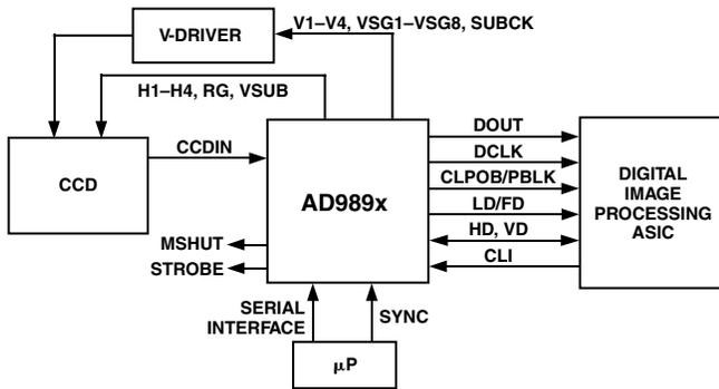
Figure 5. Typical System Block Diagram, Master Mode
