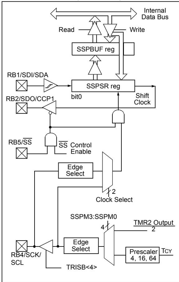
To enable the serial port, SSP enable bit SSPEN (SSPCON<5>) must be set. To reset or reconfigure SPI mode, clear bit SSPEN, re-initialize the SSPCON register, and then set bit SSPEN. This configures the SDI, SDO, SCK, and SS pins as serial port pins. For the pins to behave as the serial port function, they must have their data direction bits (in the TRISB register) appropriately programmed. That is:
