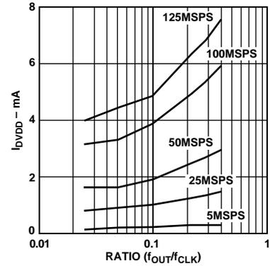
Figure 21.  $I_{DVDD}$  vs. Ratio @  $DVDD = 3\text{ V}$
