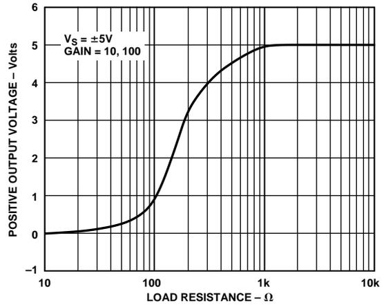
Figure 4. Positive Output Voltage Swing vs. Resistive Load
