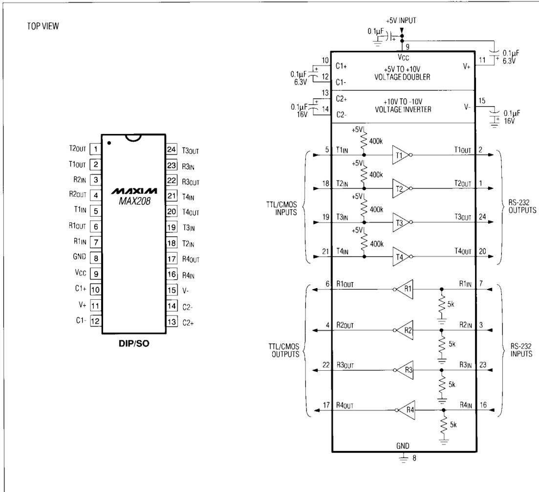
Figure 14. MAX208 Pin Configuration and Typical Operating Circuit
