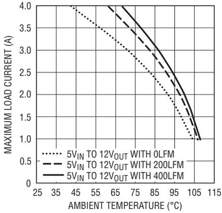
Figure 7. 5V<sub>IN</sub> to 12V<sub>OUT</sub> without Heatsink
