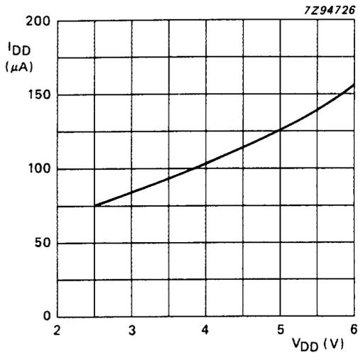
(a) Internal oscillator;  $T_{amb} = +27\text{ }^{\circ}\text{C}$ .
