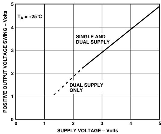
Figure 2. Positive Output Voltage Swing vs. Supply Voltage
