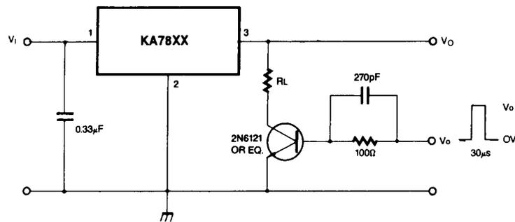
Fig. 7 Ripple Rejection
