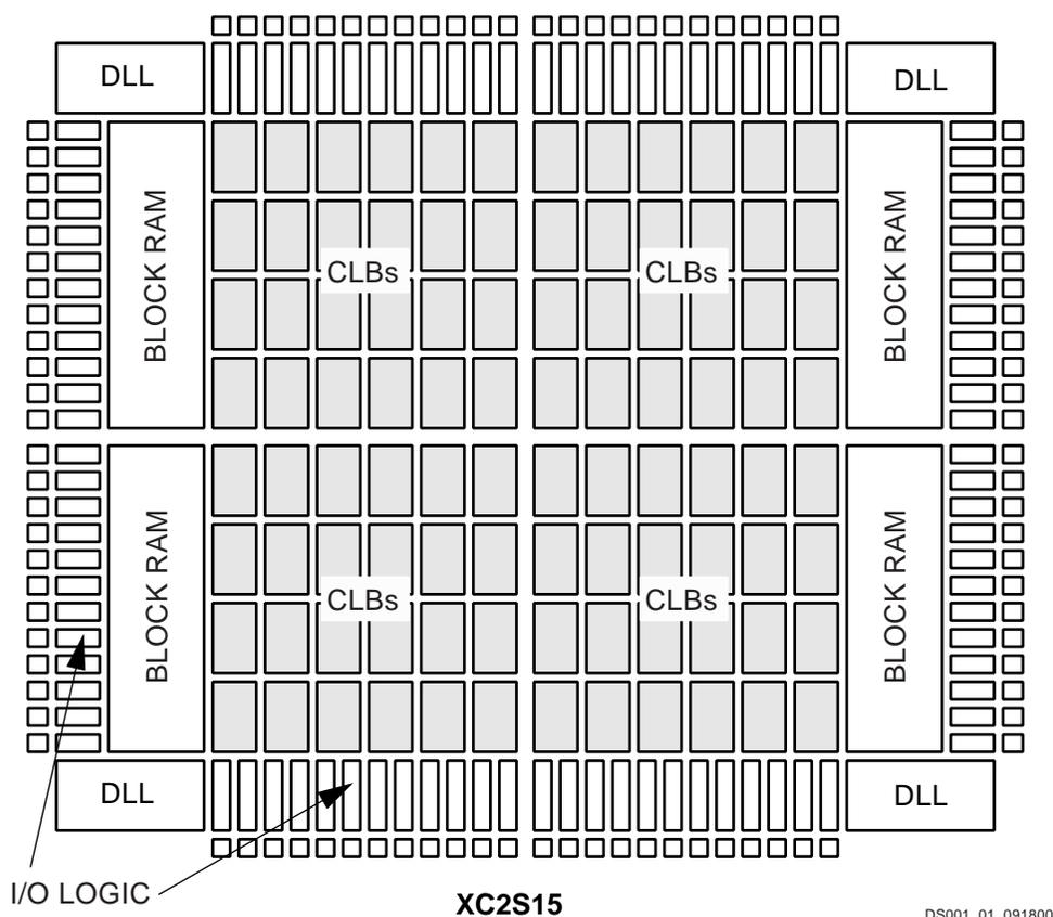
Figure 1: Basic Spartan-II Family FPGA Block Diagram
