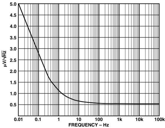
Figure 19. Voltage Noise Spectral Density vs. Frequency
