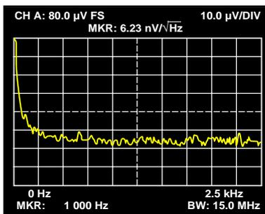
Voltage Noise Density vs. Frequency
