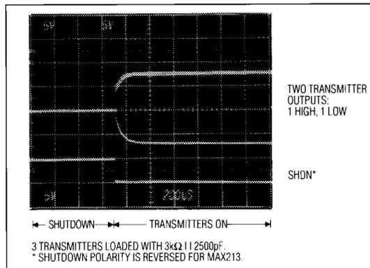
Figure 5. Transmitter Outputs When Exiting Shutdown
