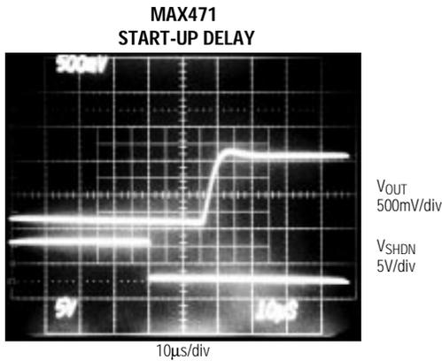
$I_{LOAD} = 1\text{A}$ ,  $R_{OUT} = 2k\Omega$  1%
