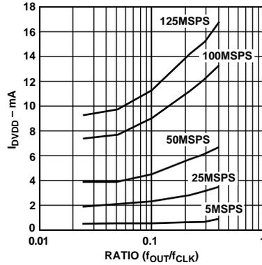
Figure 20.  $I_{DVDD}$  vs. Ratio @  $DVDD = 5\text{ V}$
