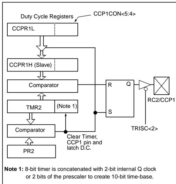
A PWM output (Figure 7-4) has a time base (period) and a time that the output stays high (on-time). The frequency of the PWM is the inverse of the period (1/period).
