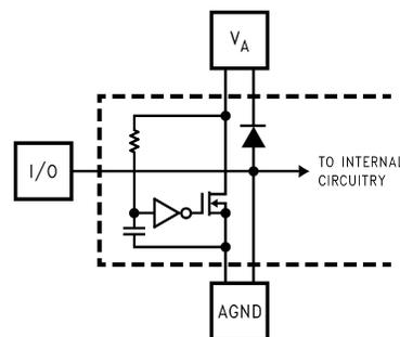
**Note 8:** To guarantee accuracy, it is required that  $V_A$  and DR  $V_D$  be well bypassed. Each supply pin must be decoupled with separate bypass capacitors.
