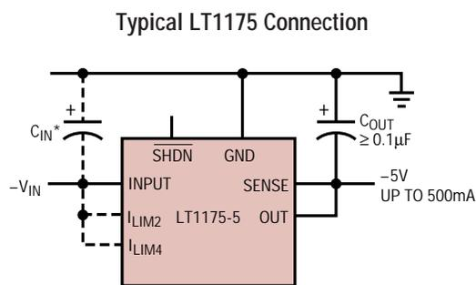
\* $C_{IN}$  IS NEEDED ONLY IF REGULATOR IS MORE THAN 6" FROM INPUT SUPPLY CAPACITOR. SEE APPLICATIONS INFORMATION SECTION FOR DETAILS
