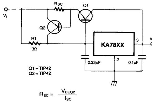
Fig. 14 Tracking Voltage Regulator
