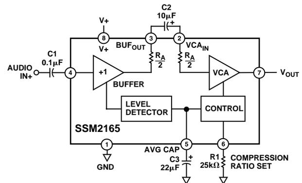
a VCA gain of 8 dB and gives  $-9.8$  dBu ( $250$  mV) before limiting. Both have a noise gate threshold of  $-64$  dBu ( $500$   $\mu\text{V}$ ), below which downward expansion reduces the gain with a ratio of approximately 1:3. That is, a  $-3$  dB reduction of output signal occurs with a  $-1$  dB reduction of input signal. For applications requiring adjustable noise gate threshold, VCA gain up to 18 dB, and adjustable rotation point, please refer to the SSM2166.
