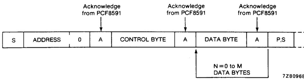
Fig.15 Bus protocol for write mode, D/A conversion.
