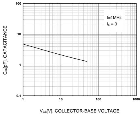
Figure 5. Output Capacitance
