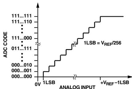
Figure 7. Transfer Characteristic
