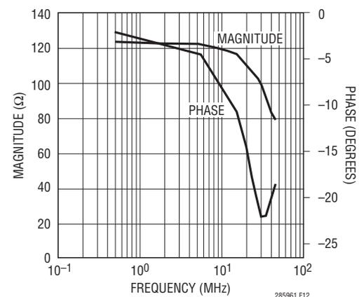
**Figure 12. Termination Magnitude and Phase vs Frequency**
