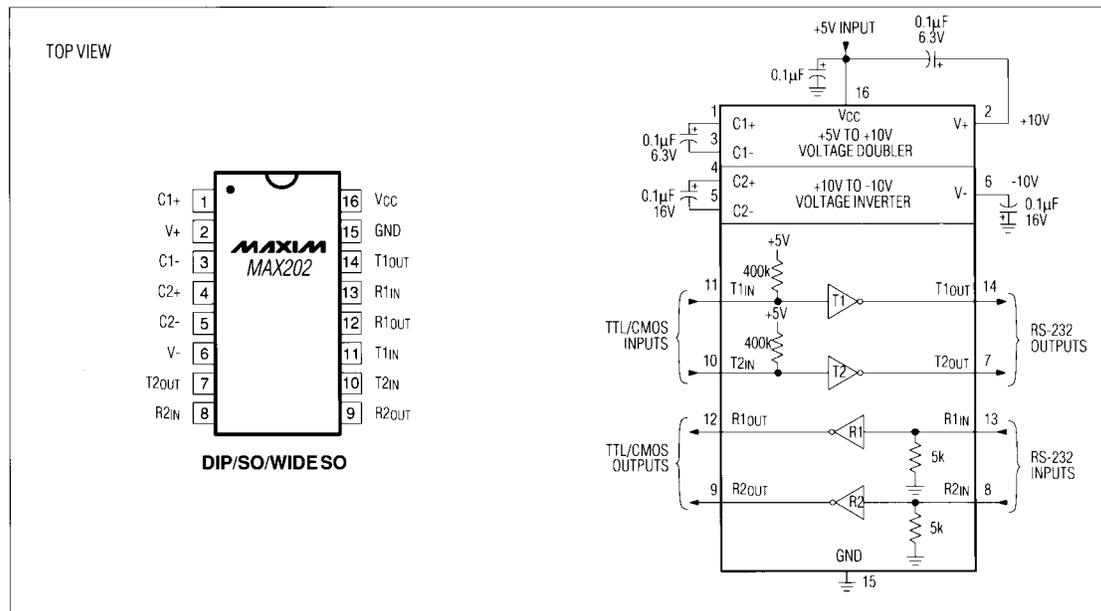
Figure 8. MAX202 Pin Configuration and Typical Operating Circuit
