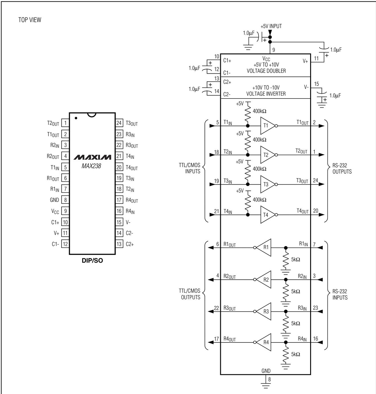
Figure 16. MAX238 Pin Configuration and Typical Operating Circuit
