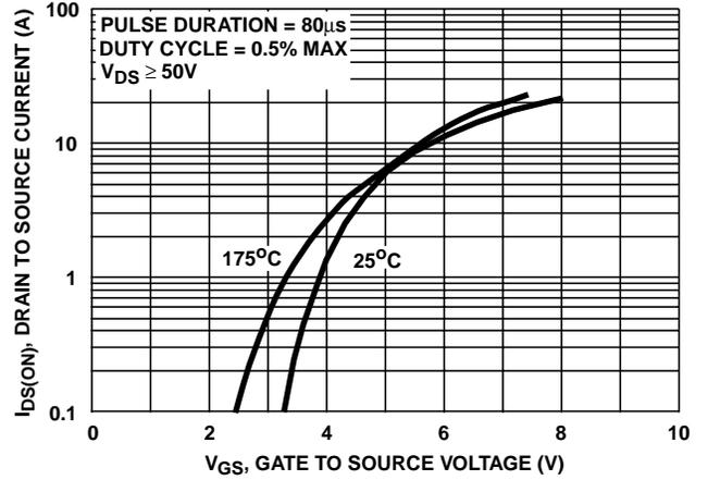
FIGURE 7. TRANSFER CHARACTERISTICS
