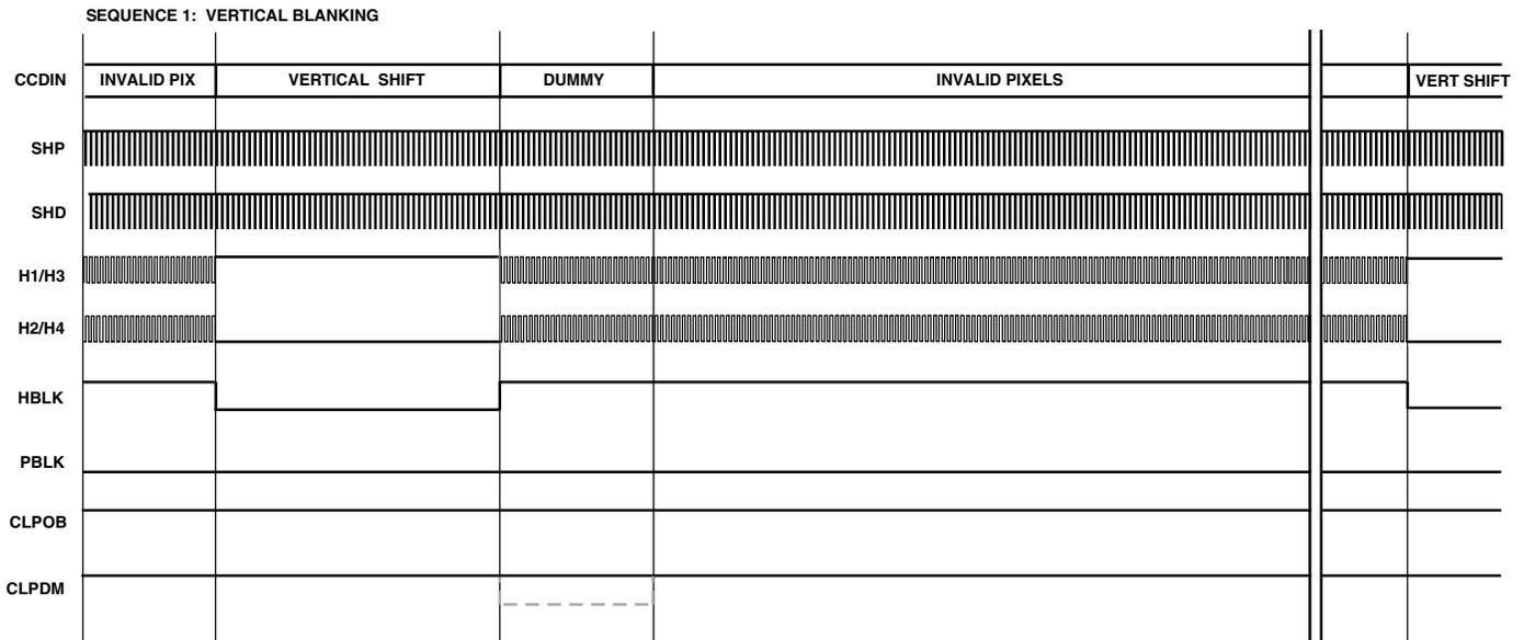
CLPDM PULSE MAY BE USED DURING HORIZONTAL DUMMY PIXELS IF THE H-CLOCKS ARE USED DURING VERTICAL BLANKING.
