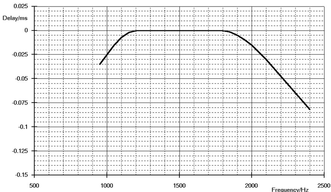
Figure 3 Rx Equaliser Group Delay (RXEQ = '1') wrt 1700Hz
