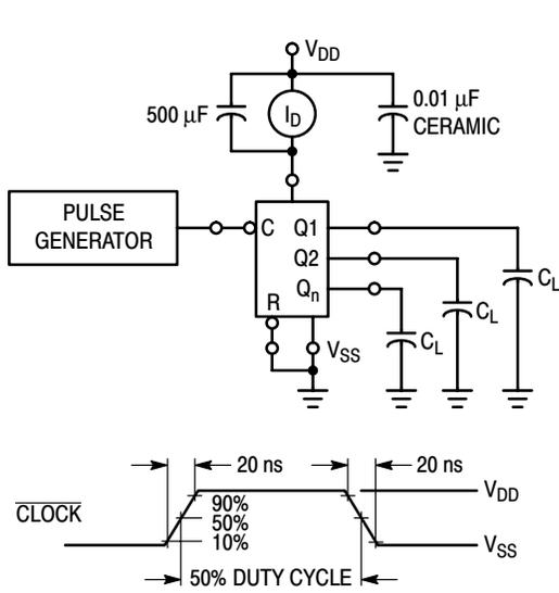
Figure 1. Power Dissipation Test Circuit and Waveform
