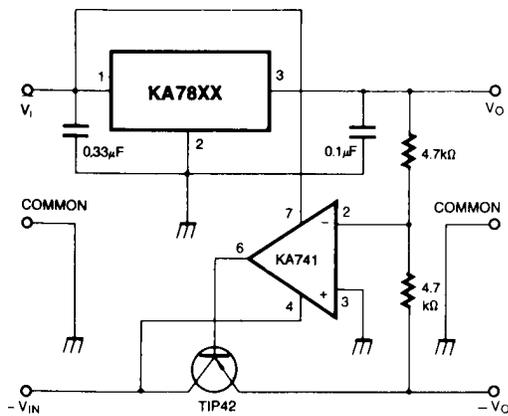
Fig. 15 Split Power Supply (±15V-1A)
