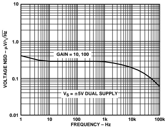
Figure 15. Noise Voltage Spectral Density vs. Frequency
