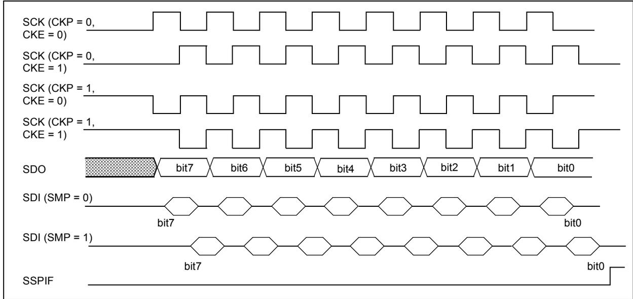
**FIGURE 10-3: SPI MODE TIMING (SLAVE MODE WITH CKE = 0)**
