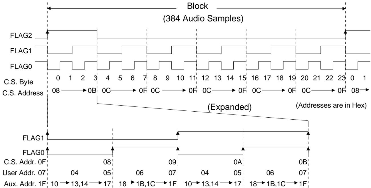
**Figure 13. CS8413 Buffer Memory Write Sequence - MODE 1**
