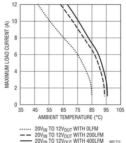
Figure 12. 20V<sub>IN</sub> to 12V<sub>OUT</sub> with Heatsink
