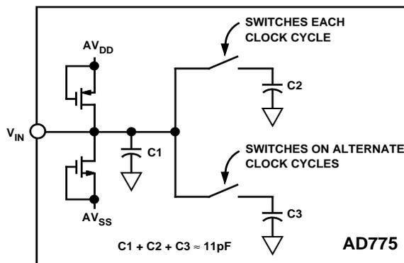
Figure 12. Equivalent Analog Input Circuit ( $V_{IN}$ )
