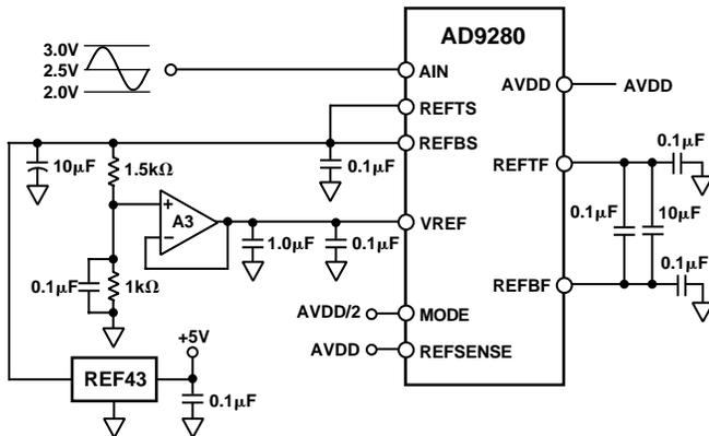
Figure 22. External Reference Mode—1 V p-p Input Span 2.5 V<sub>CM</sub>
