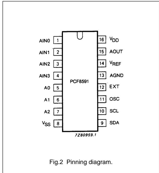
Fig.2 Pinning diagram.
