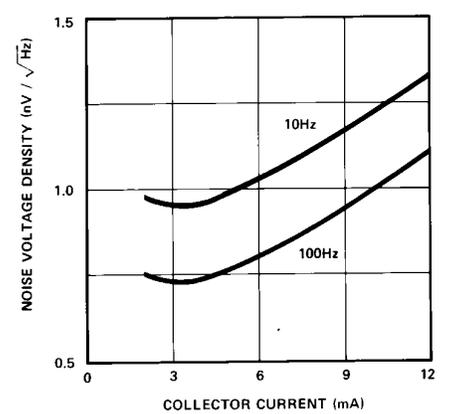
Figure 9. Noise Voltage Density vs. Collector Current
