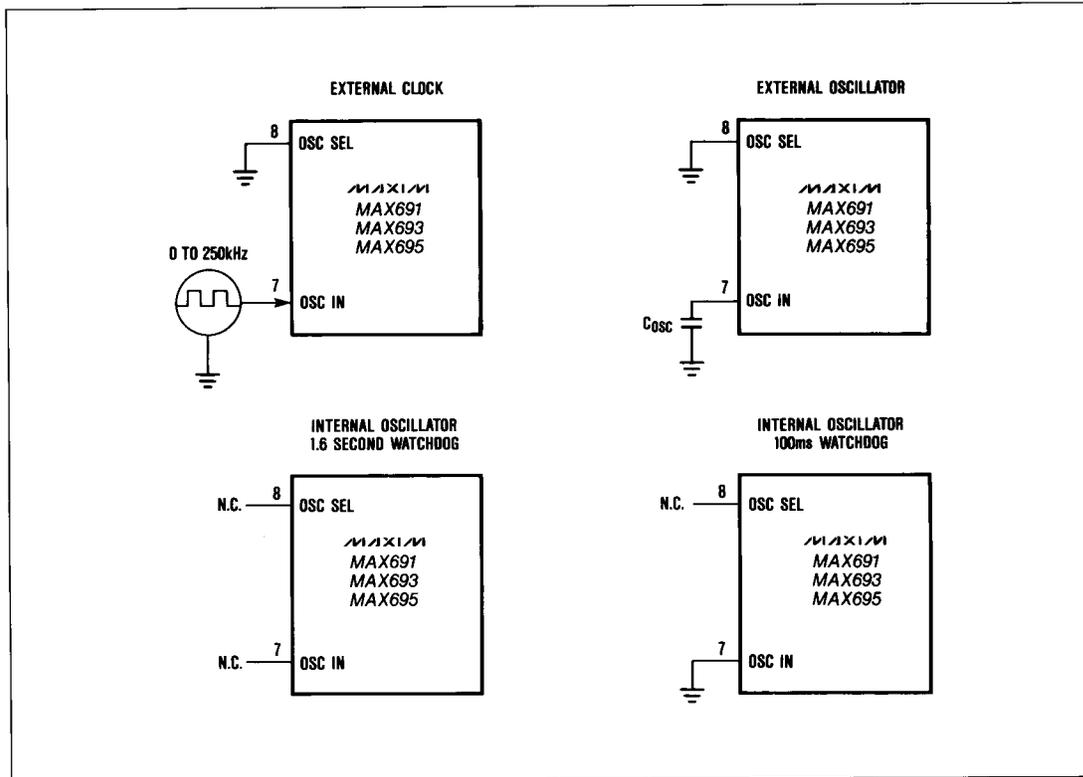
Figure 8. Oscillator Circuits
