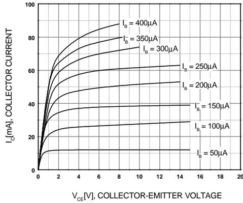
Figure 1. Static Characteristic
