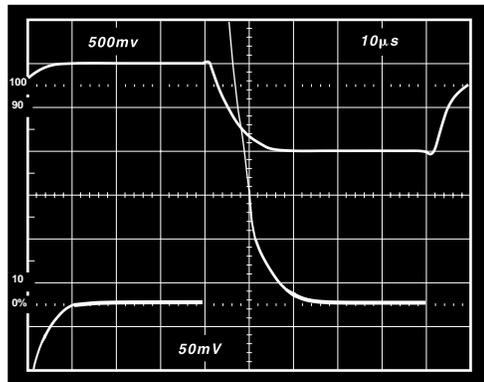
Figure 24. Settling Time.  $V_S = \pm 5\text{ V}$ ,  $G = 100$
