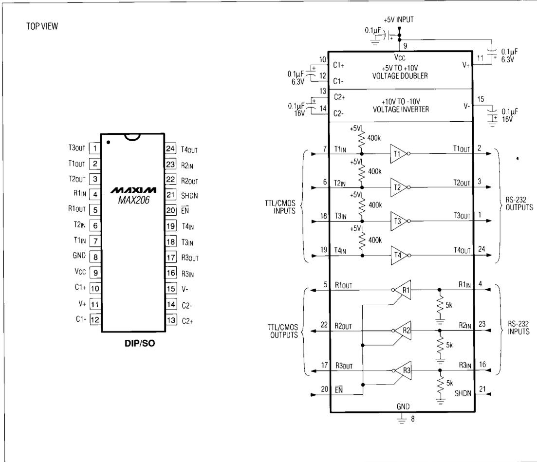
Figure 12. MAX206 Pin Configuration and Typical Operating Circuit
