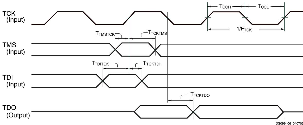
Figure 8: JTAG Waveforms
