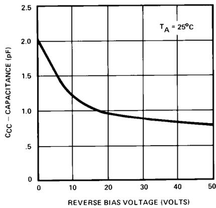
Figure 16. Collector-to-Collector Capacitance vs. Reverse Bias Voltage
