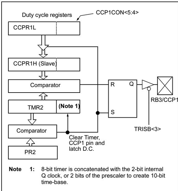
A PWM output (Figure 11-3) has a time-base (period) and a time that the output stays high (duty cycle). The frequency of the PWM is the inverse of the period (1/period).
