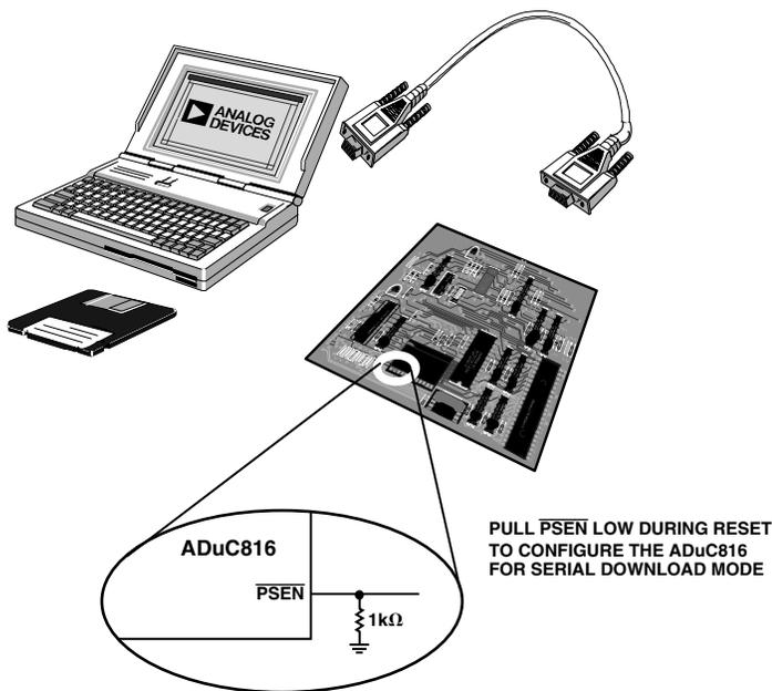
Figure 27. Flash/EE Memory Serial Download Mode Programming
