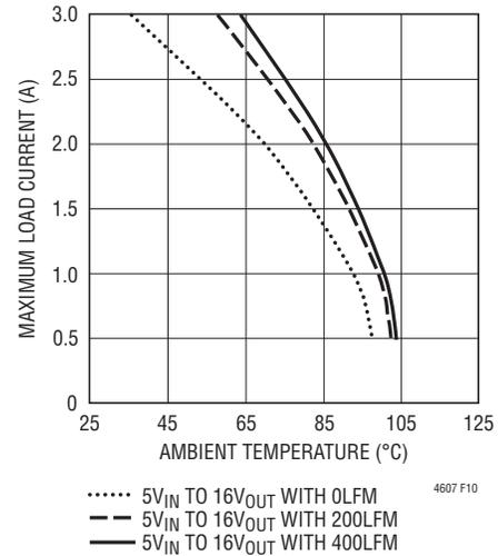
Figure 10. 5V<sub>IN</sub> to 16V<sub>OUT</sub> with Heatsink
