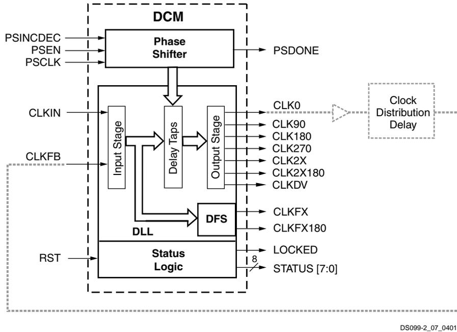
Figure 13: DCM Functional Blocks and Associated Signals
