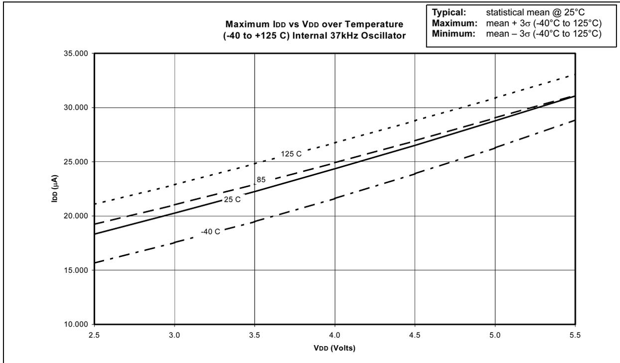
**FIGURE 18-25: TYPICAL I<sub>DD</sub> VS V<sub>DD</sub> OVER TEMPERATURE (-40 TO +125°C) INTERNAL 37 kHz OSCILLATOR**
