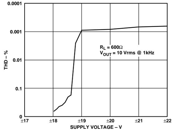
Figure 5. THD + Noise vs. Supply Voltage
