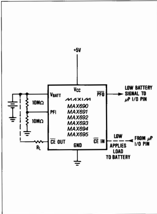
Figure 11. Backup Battery Monitor with Optional Test Load
