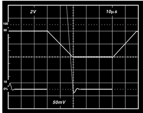
Figure 23. Settling Time.  $V_S = \pm 5\text{ V}$ ,  $G = 10$
