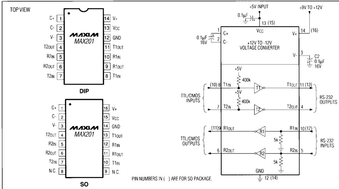
Figure 7. MAX201 Pin Configurations and Typical Operating Circuit
