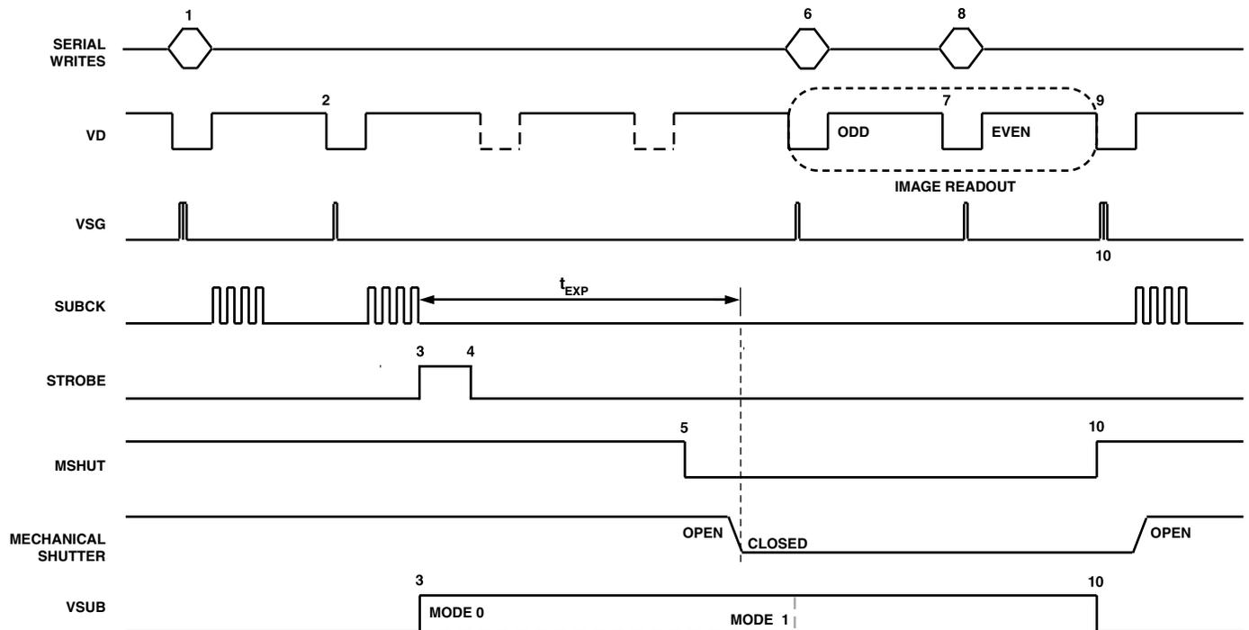
Figure 35. Exposure and Readout of Interlaced Frame
