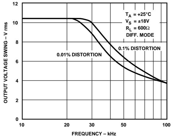
Figure 4. Maximum Output Voltage Swing vs. Frequency
