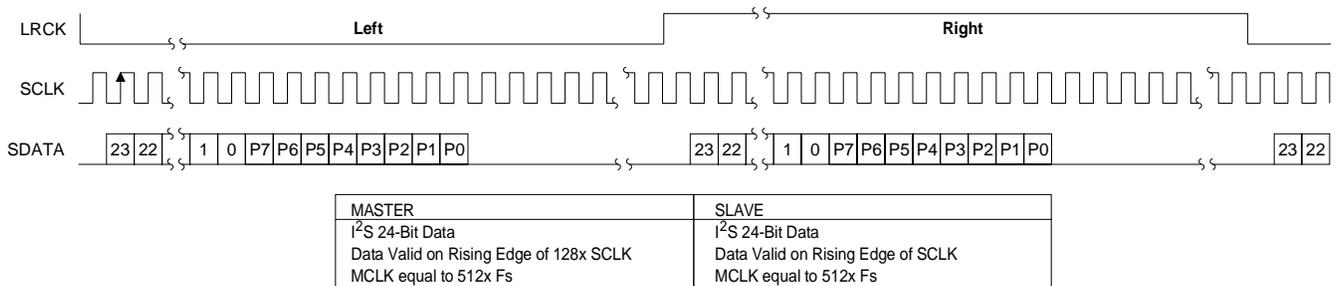
**Figure 7. Control Port Mode, Serial Data. I<sup>2</sup>S Compatible. 128x Oversampling Mode.**
