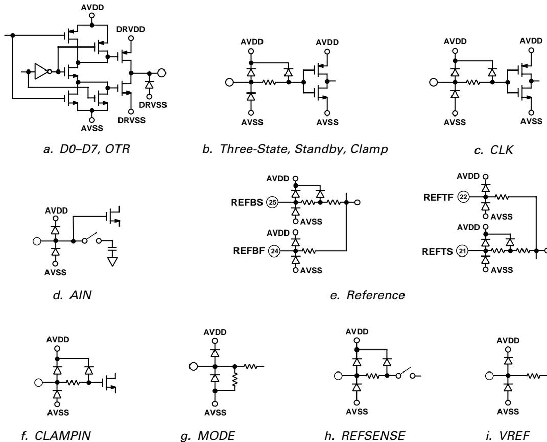
Figure 2. Equivalent Circuits
