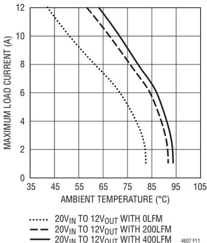
Figure 11. 20V<sub>IN</sub> to 12V<sub>OUT</sub> without Heatsink
