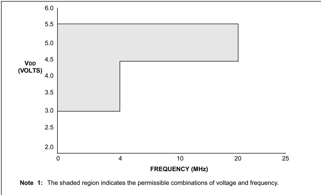
**FIGURE 17-3: PIC16LF62X VOLTAGE-FREQUENCY GRAPH,  $0^{\circ}\text{C} \leq \text{TA} \leq +70^{\circ}\text{C}$**
