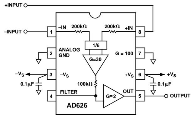
Figure 30. AD626 Configured for a Gain of 100
