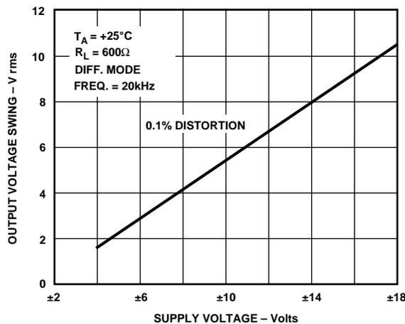
Figure 5. Output Voltage Swing vs. Supply Voltage
