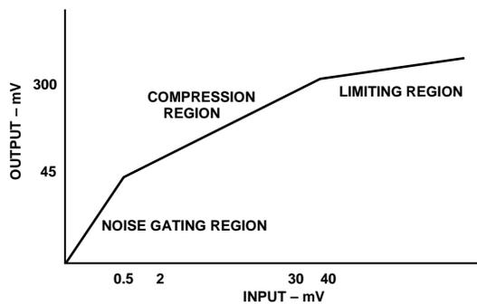
Figure 10. Transfer Characteristic
