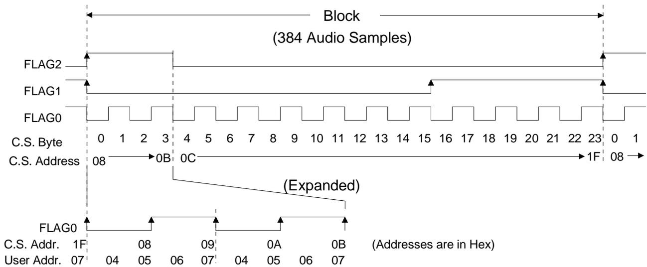
**Figure 12. CS8413 Buffer Memory Write Sequence - MODE 0**
