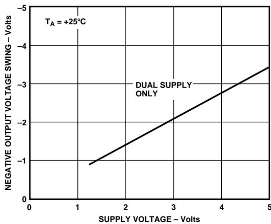
Figure 3. Negative Output Voltage Swing vs. Supply Voltage
