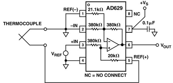
Figure 36. A Gain of 19 Thermocouple Amplifier
