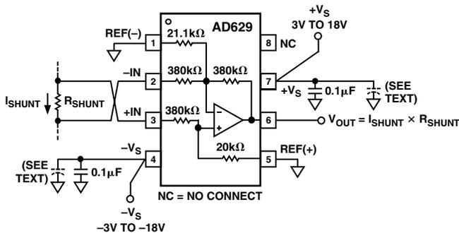
Figure 29. Basic Connections
