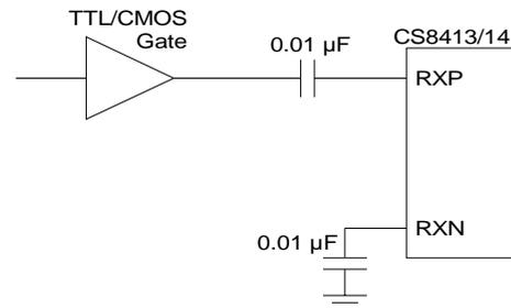
Figure 24. TTL/CMOS Interface
