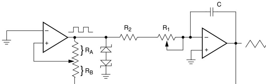
$$\text{frequency} \propto R_1, R_2, C$$
