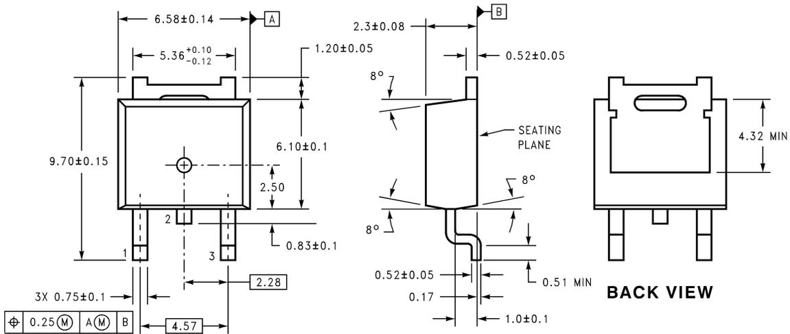
**DIMENSIONS ARE IN MILLIMETERS**
