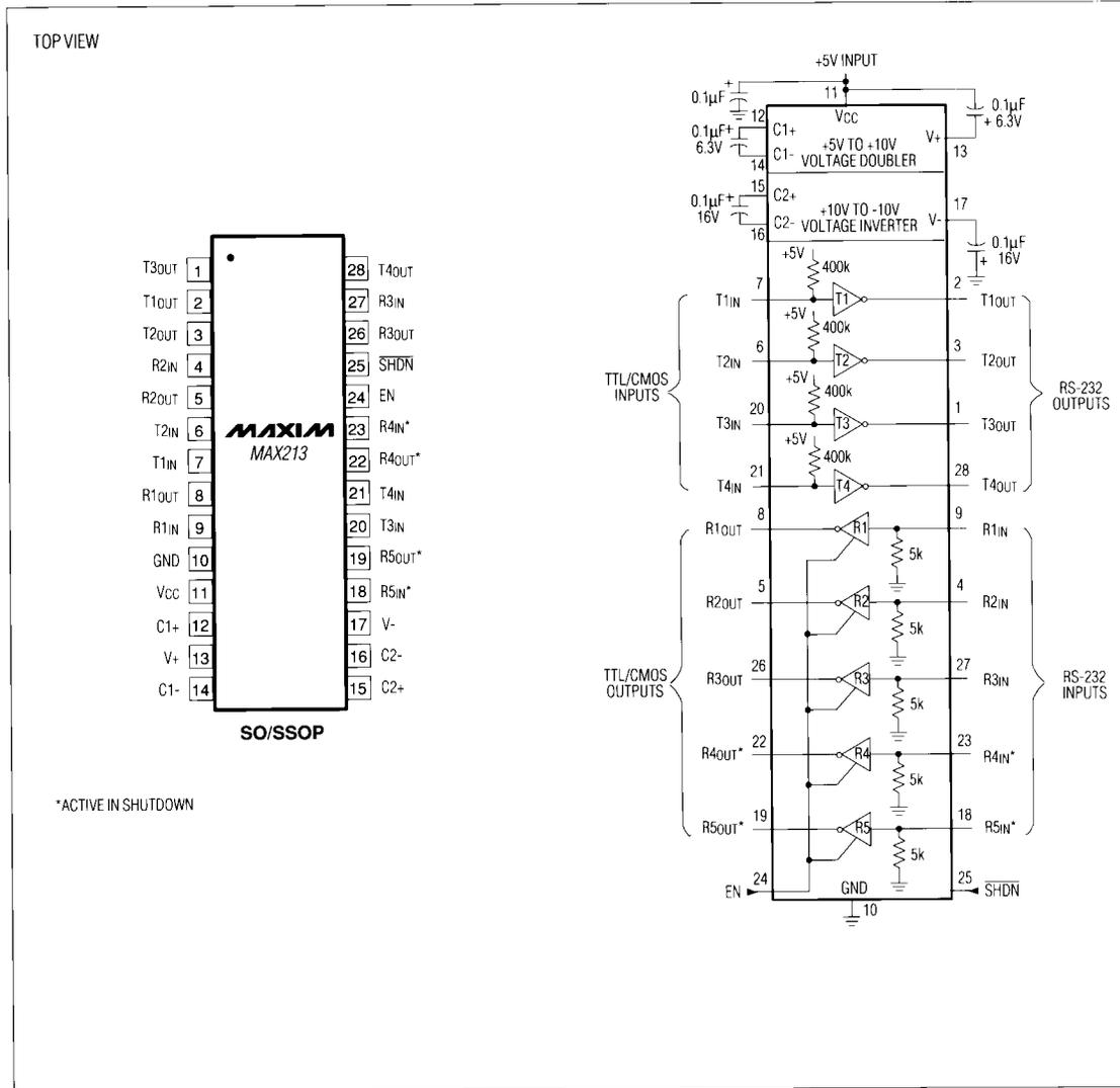
Figure 17. MAX213 Pin Configuration and Typical Operating Circuit
