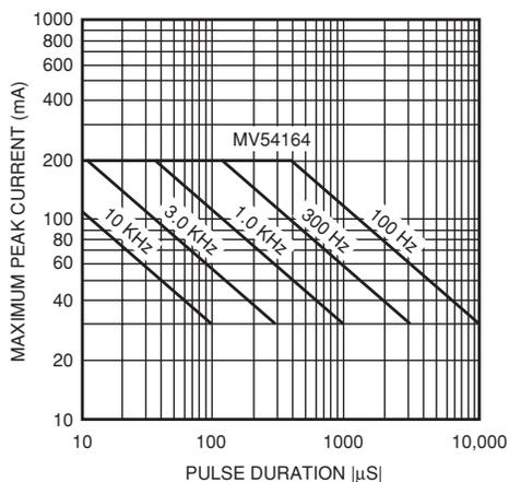
**Fig. 5. Maximum Peak Current vs. Pulse Duration**
