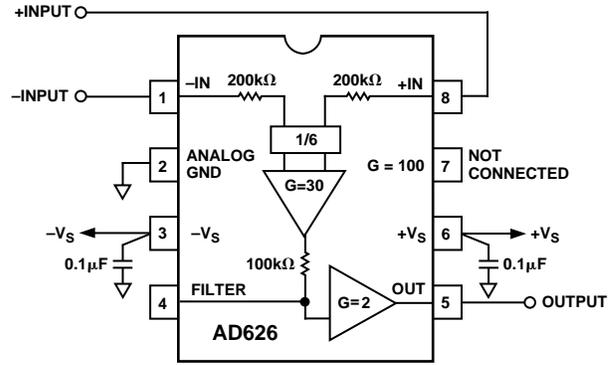
Figure 29. AD626 Configured for a Gain of 10
