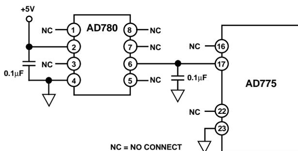
Figure 10. Reference Configuration: 0 V to 2.5 V
