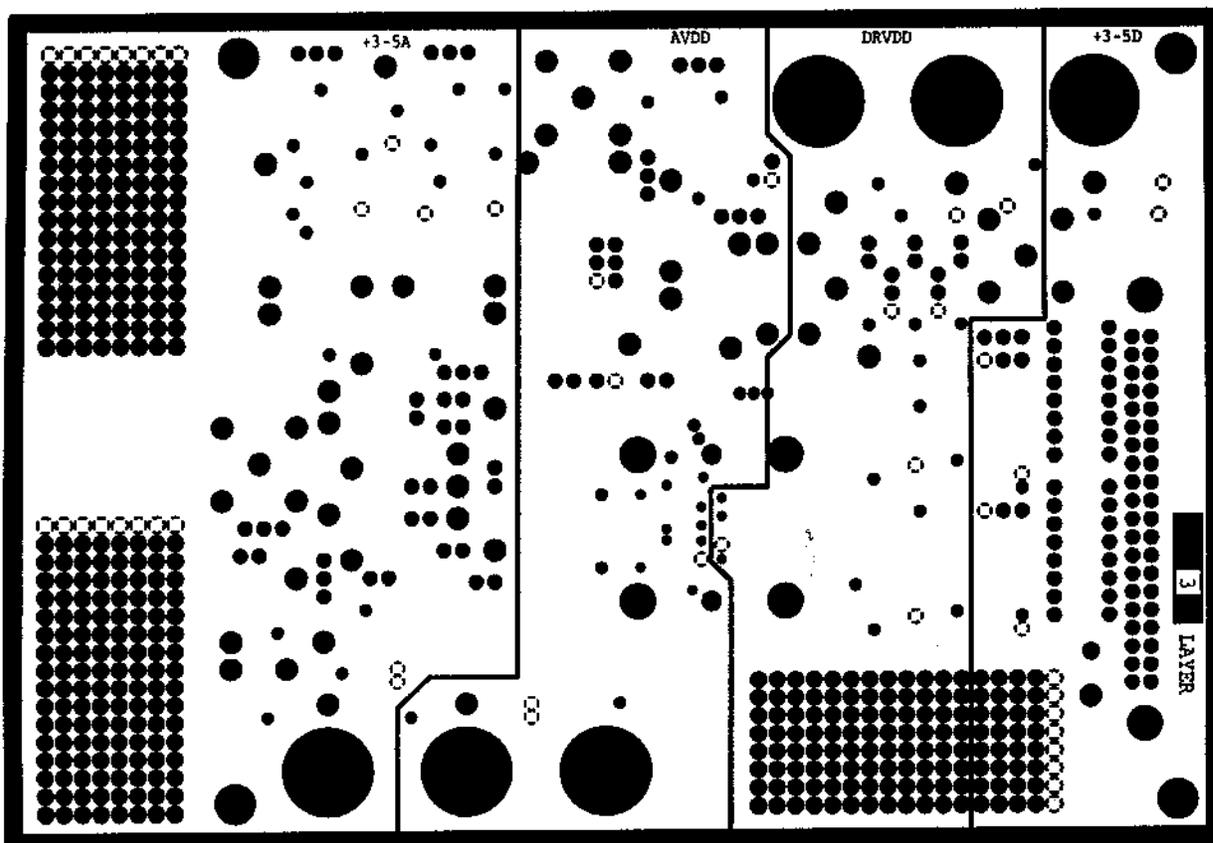
Figure 40c. Evaluation Board Power Plane (Not to Scale)
