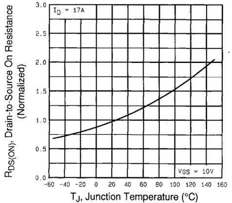
**Fig 4.** Normalized On-Resistance
