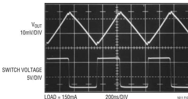
**Figure 10. 22µF “B” Case Tantalum Capacitor (AVX TAJ “B” Series) Has ESR Resulting in 20mV<sub>p-p</sub> Voltage Ripple at Output**
