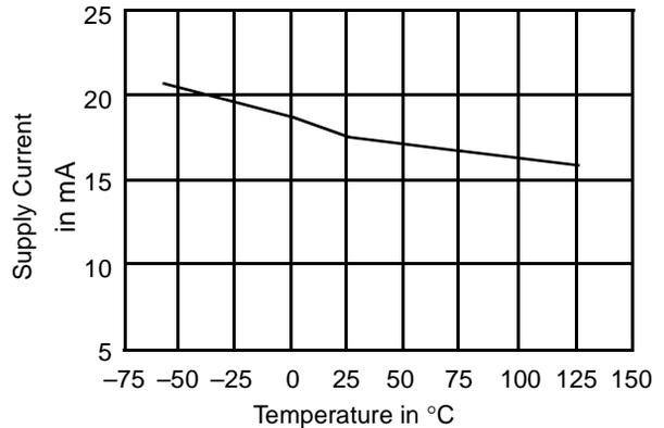
**Figure 2. Typical Supply Current vs. Temperature**
